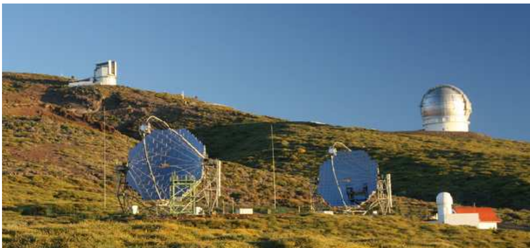
Figure 2.1: The MAGIC stereoscopic system of telescopes. On the left, the first MAGIC telescope that has been operating since 2003 and now faces the fourth cycle of scientific observation. On the right, the second MAGIC telescope, currently under commissioning. While the structures of the two telescopes are very similar, all MAGIC II subsystems are substantially ameliorated to the advantage of the overall performance. Picture from R. Wagner.
