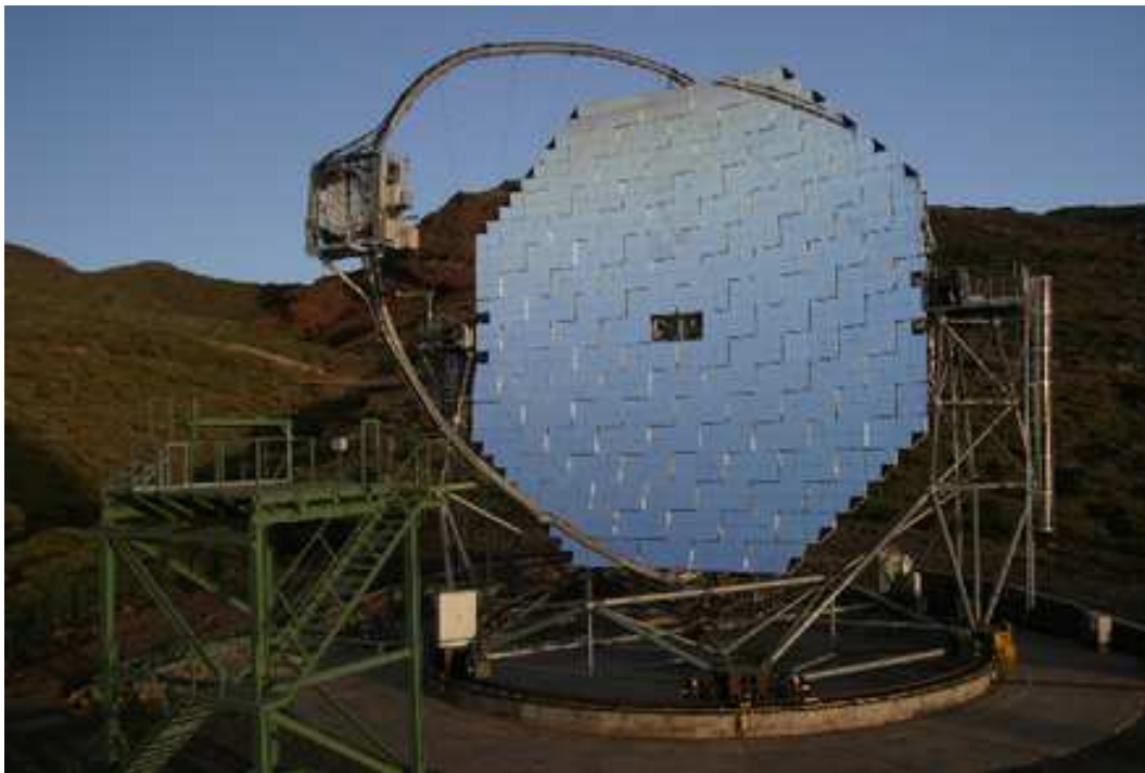
Figure 2.2: The first MAGIC telescope. The reflector dish has a 17 m diameter and the camera is placed at a distance of 17 m ( f/D = 1 ). The reflector is tessellated and composed by 956 mirrors of 0.5 \times 0.5 \text{ m}^2 area. The camera weighs \simeq 0.5 tons and contains the 576 photomultipliers and the optical converter that transmit the signal through a 160 m optical fibre. The structure is a CFRP space-frame plus some aluminum parts for connections and bearings. The structure is mounted alt-azimuthally and rotates on a 18 m diameter rail. More details are in the text. Picture from R. Wagner.
