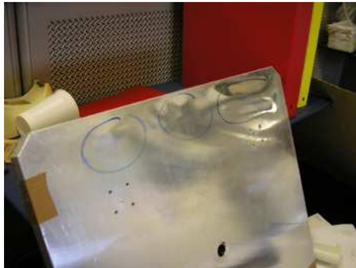
Figure 4.5: A damaged mirror from MAGIC I. The bubble created by the internal accumulation of water condensing into ice is clearly visible on the back side.
