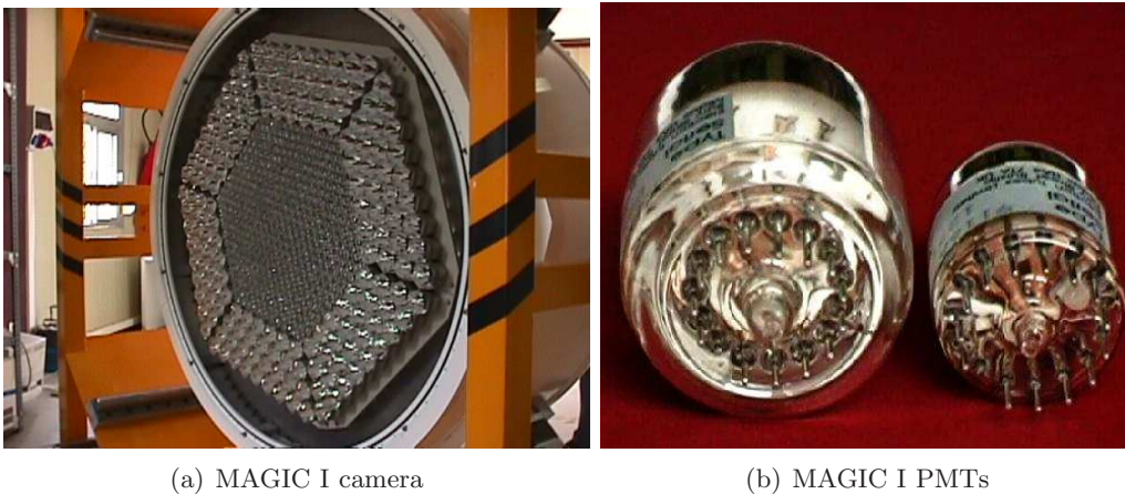
Figure 2.4: The camera system of MAGIC I. In figure (a), the camera before shipment. Inner and outer pixels, shown in figure (b), are mounted. The light-catchers (Winston-cones) are also mounted in front of the pixels. In figure (b), the two types of Electron Tubes PMT are shown. The larger one (1.5' \varnothing ) is mounted on the outermost part of the camera, the smaller pixels (1' \varnothing ) are mounted in the central part.
