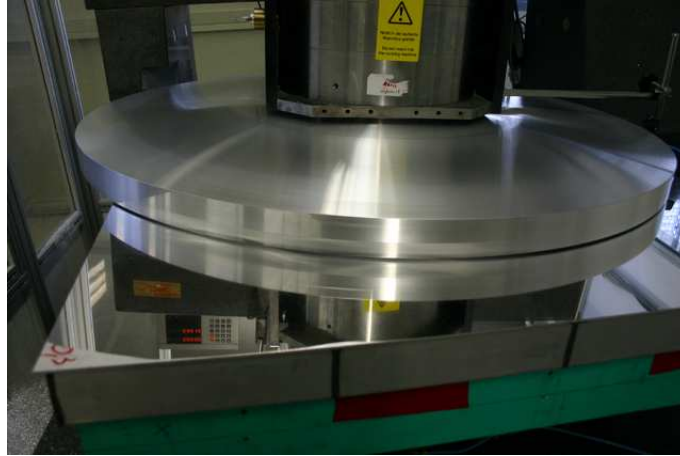
Figure 4.13: A sketch of the LT-Ultra machine used to diamond-mill MAGIC II mirrors.
