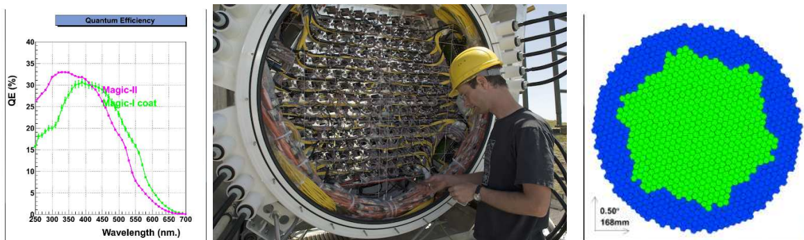
Figure 2.5: The MAGIC II camera, trigger and photomultipliers photocathode efficiency.
