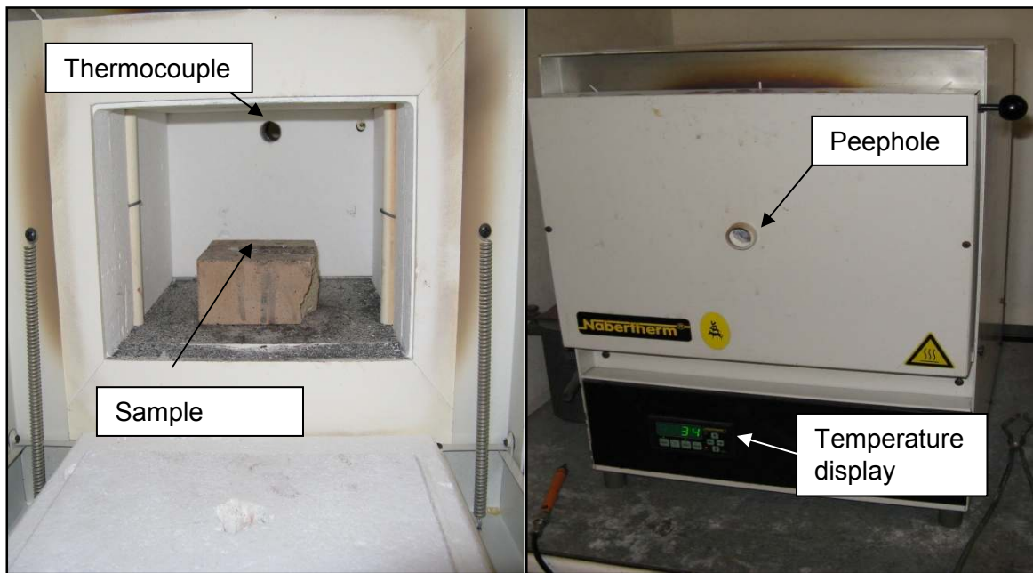
Fig. 7 Test device; inner of the muffle furnace with sample position and internal thermocouple position indicated
