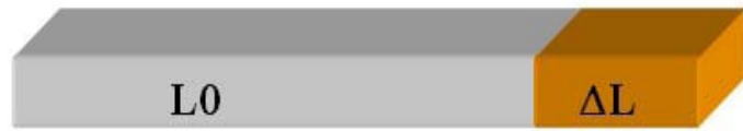
Fig 1.10: Strain of a one-dimensional object is limited to lengthening or shortening. Strain ( \epsilon ) is the deformation of an object relative to its original shape: \epsilon = (L - L^0) / L^0 ; L = final length; L^0 = original length (from 30, Teske AJ et al. 2007).
