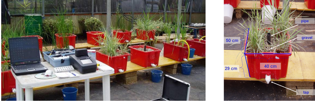
Figure 30 - General view of the experimental set up and detail of a tank
