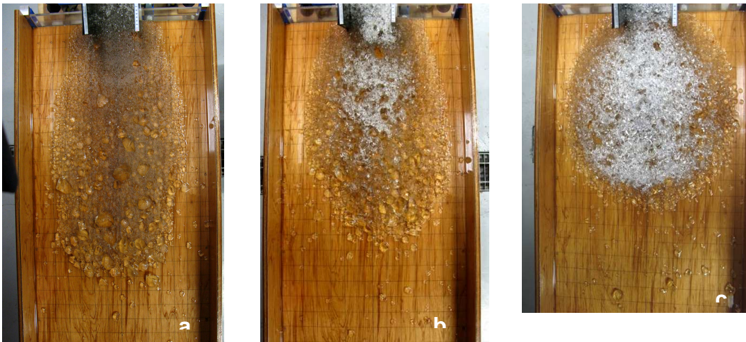
Figure 6-5 Test depositions for PSDs with different C_U : a) PSD9-mod ( C_U=20.2 ); b) PSD11-up ( C_U=9.8 ); c) PSD16-up ( C_U=3.3 )
