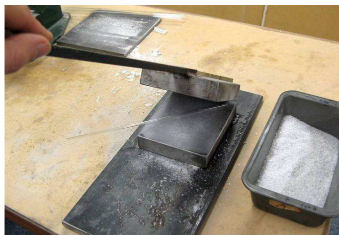
Figure 4-12 Steel slabs used for crushing the glass tubing
