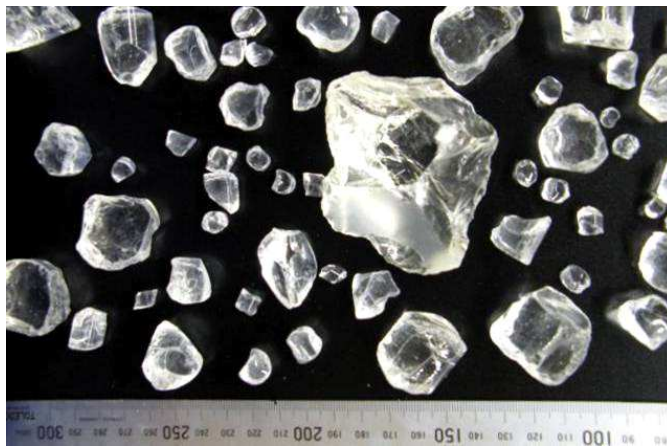
Figure 4-13 Coarse glass particles used as transparent solid
