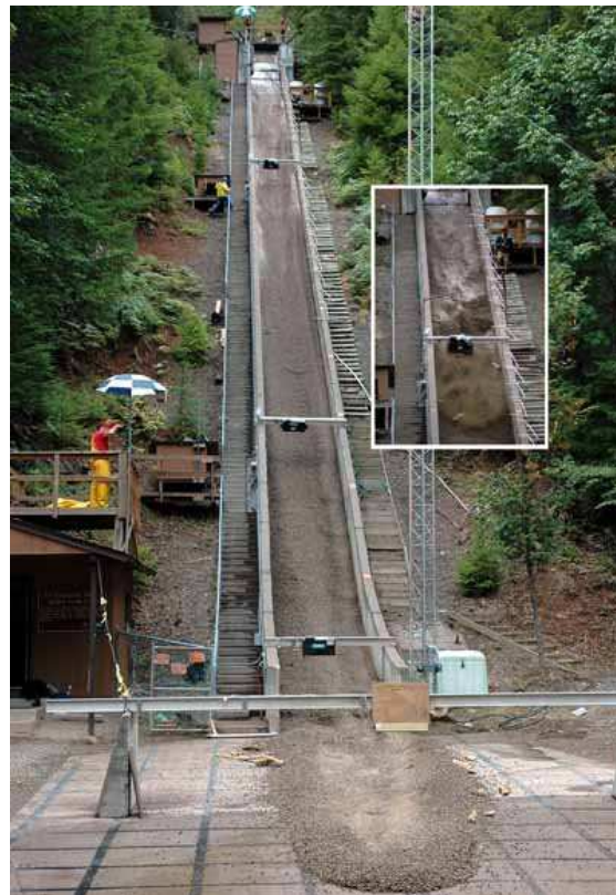
Figure 1-8 U.S. Geological Survey large-scale debris flow flume (Logan and Iverson, 2007)
