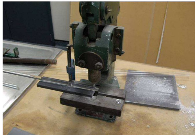
Figure 4-11 Bench machine used to produce the larger particles by cutting the glass rods
