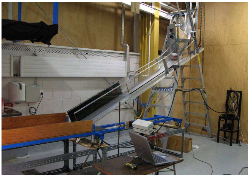
Figure 4-19 Experimental set up with the laser line generator lens beneath the flume
