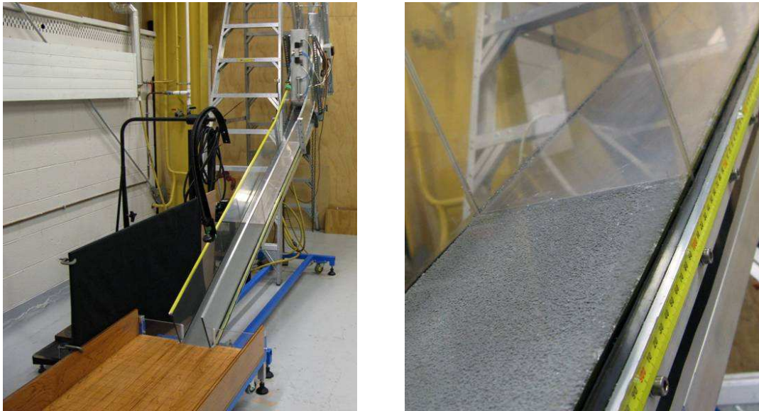
Figure 4-16 Set up of the flume with the laser from the top and particular of the different material on the bed of the channel (steel surface at the first half and synthetic rough material in the last 1m portion)
