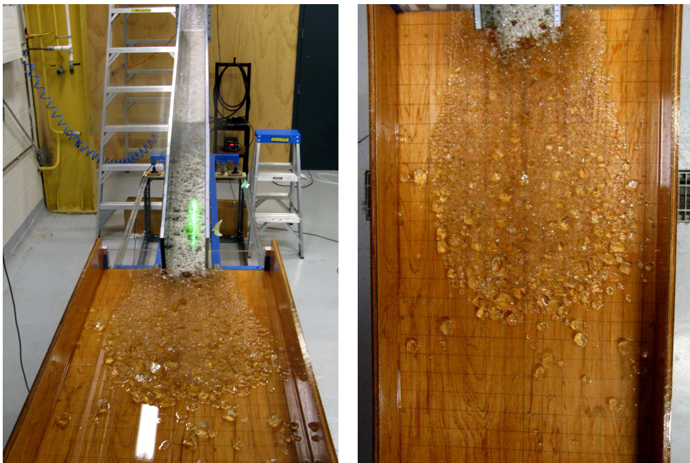
Figure 4-26 Typical deposit at the base of the slope
