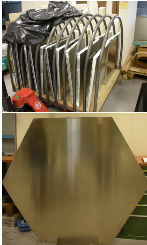
Figure 4.21: Images of mirror substrates of different dimensions. Top: Several small substrates with MAGIC I dimensions. Bottom: Substrate with LST dimension.
