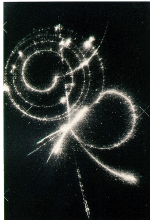
Figure 1.3: Tracks captured a streaming chamber indicating a pion (looping track to the right from a collision at the center of the image) and muon (four anticlockwise curls in the upper left corner) decay.
