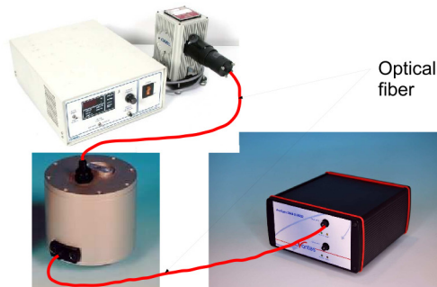
Figure 5.5: Equipment for measuring the spectral reflectance locally on the mirror surface. The Avaspec spectrophotometer and the Oriol light source are connected via optical fibers.
