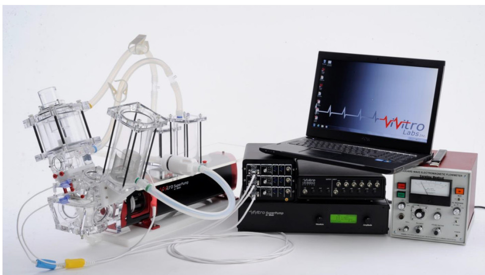
Fig.1.13 ViVITRO pulse duplicator system, acquisition and control dock station and laptop, and the Carolina Medical Inc. electromagnetic flowmeter.
