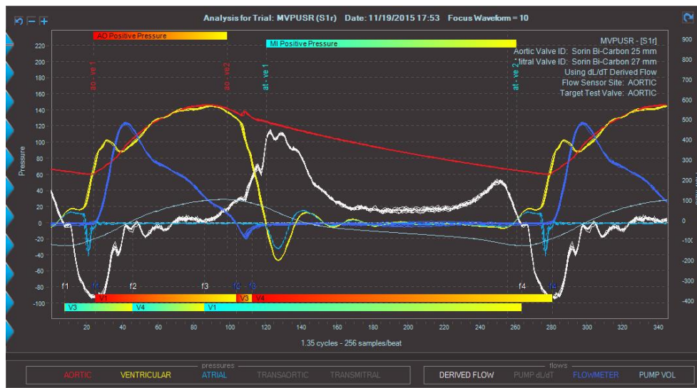
Fig.4.6 Mean pressures ( p_v , yellow line; p_{ao} , red line) and flow (upstream aortic valve, blue line) trends for Sorin Bi-Carbon 25 mm obtained with ViVitro superpump.
