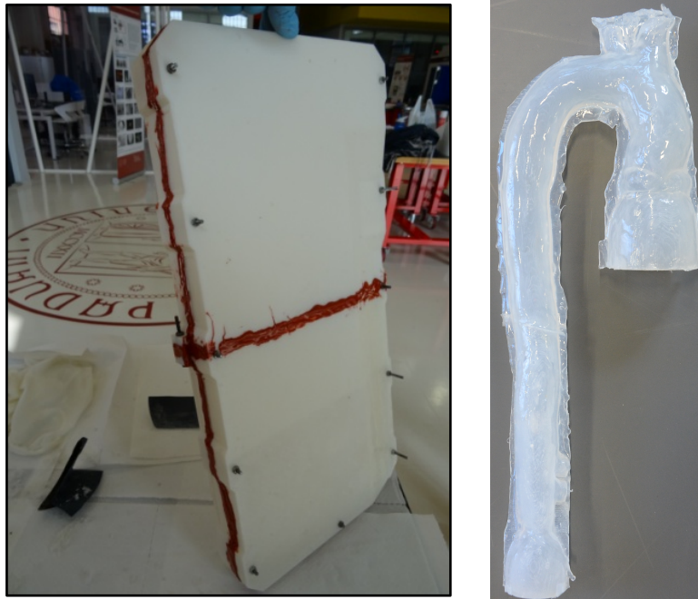
Fig.3.34 Sealed close mould in which the silicone has been casted, and the final silicone aortic arch.
