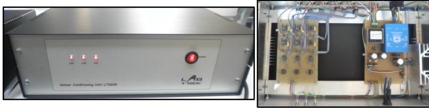
Fig.3.12 Signals conditioning unit, box and inside circuits for filtering and amplification.
