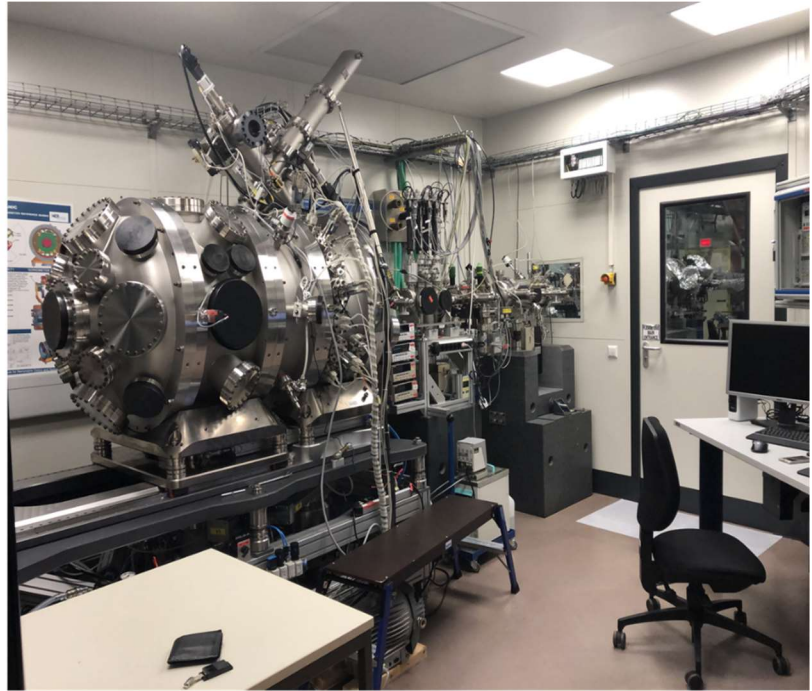
Figure 3.13 Optics beamline at Bessy II synchrotron. In the left pics, the positioning of the samples can be appreciated, the holder used have 3 holes, one for measuring the direct light and the other 2 for samples.
