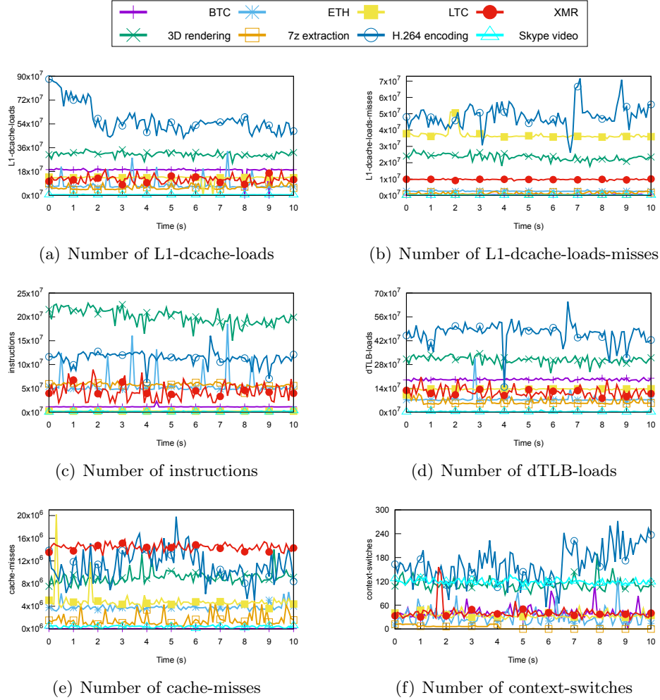
Figure 6.1: A representative example of variation in events while mining different cryptocurrencies and performing some common user-tasks. HPC were polled every 100ms. The line-points in the graphs do not represent data points and are merely used to make lines distinguishable.
