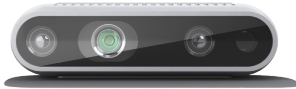
Fig. 2.4: Intel RealSense DS435, an example of commercial active stereo system. [20]
