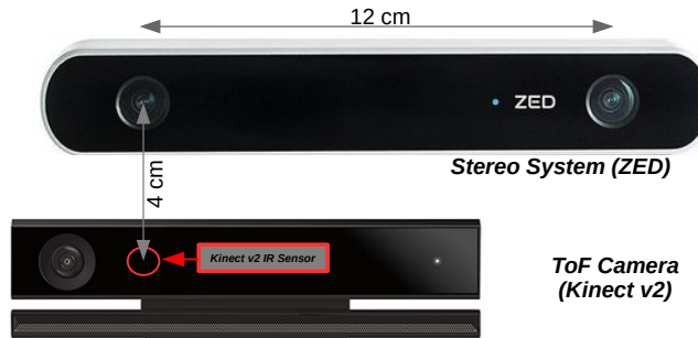
Fig. 3.3: Representation of the real Stereo-ToF acquisition system used for the REAL3 dataset. The figure shows the relative position of the ZED camera and of the Kinect v2.
