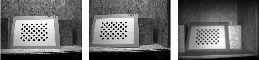
Fig. 3.6: Acquisition of the dot geometrical calibration pattern from s_0 (left), s_1 (center) and the amplitude image of the ToF camera (right).
