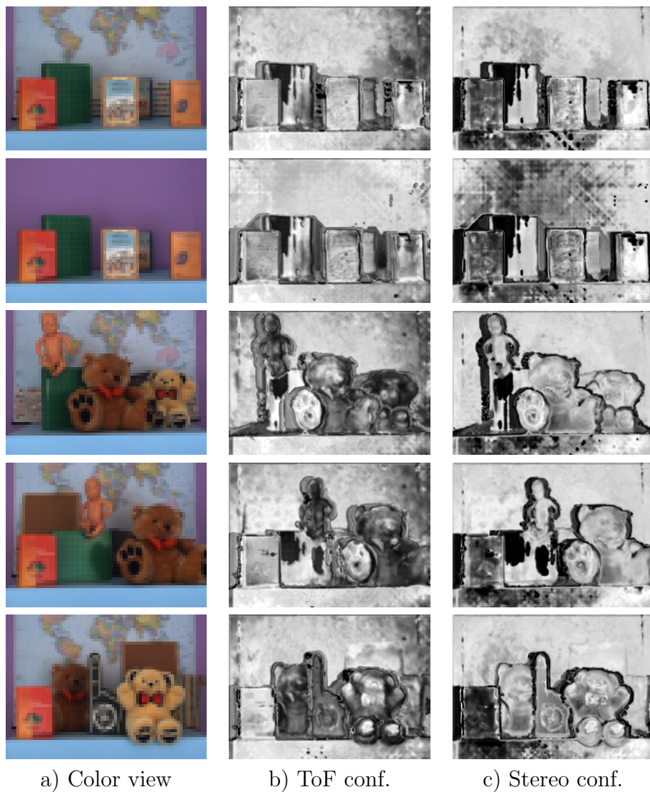
Fig. 6.7: Confidence information computed by the proposed deep learning architecture for the scenes in the LTTM5 dataset: a) Color view; b) Estimated ToF confidence; c) Estimated stereo confidence. Brighter areas correspond to higher confidence values, while darker pixels to low confidence ones.
