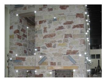
Figure A.1: URM model: detail of the damage at 0.35g.
