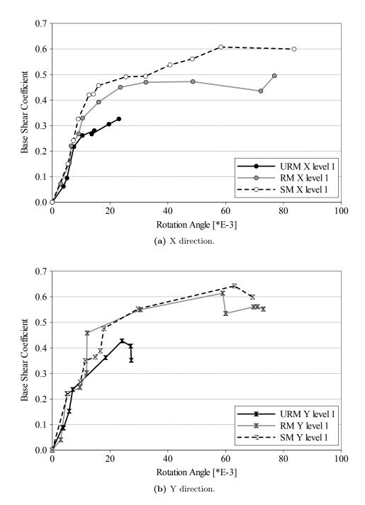
Figure 4.42: Relationships between Base Shear Coefficients and the first storey rotation angle.
