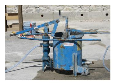
Figure 2.6: Hand pump for grout injection.
