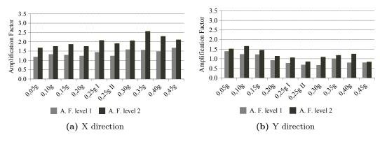
Figure 4.17: URM, trend of Amplification Factors in both directions.
