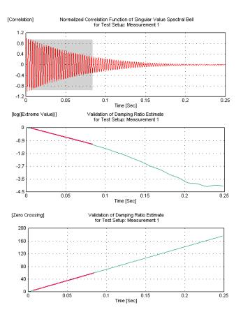
Figure 1.53: Plot of the normalized correlation function (top); damping ratio estimation from the decay of the correlation function (centre); natural frequency identification by zero-crossing counting (bottom); [Jacobsen *et al.*, 2006].
