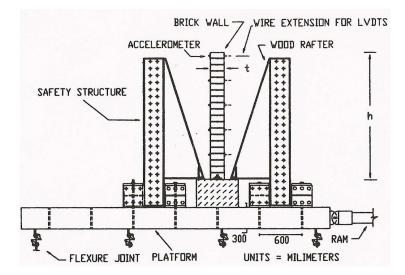
Figure 1.30: Equipment for shaking table tests [Bariola et al., 1990].
