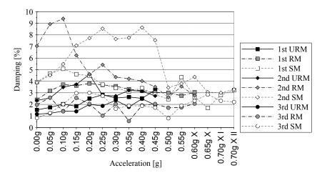
Figure 4.33: Comparison of the damping values of all building models.
