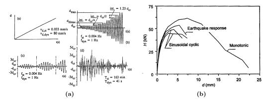
Figure 1.18: Loading patter (left) and related analyses (right) [Tomaževič et al., 1996].
