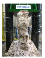
Figure 5.10: Undamaged core of specimen R7 after the test.
