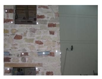
Figure A.4: URM model: detail of the damage at 0.45g.
