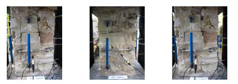
Figure 5.5: Detail of cracks in stone at the beginning of the test.
