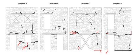
Figure 4.16: SM, crack pattern after step 0.70g in the X direction, end of experiment.
