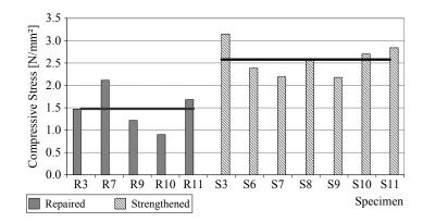
Figure 5.3: Stress levels for first crack appearance in each specimen.
