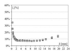
Figure 6.48: S4: Viscous damping vs displacement.
