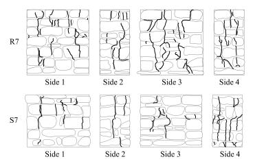
Figure 5.18: Crack pattern for R7 and S7 specimens at  $8.40N/mm^2$ .
