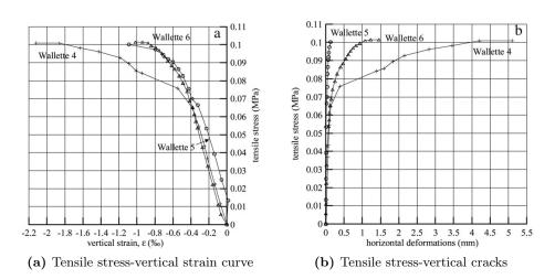
Figure 1.26: Results of diagonal compression tests [Vintzileou and Miltiadou-Fezans, 2008].
