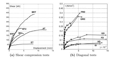
Figure 1.23: Results of specimens tested by Vignoli [Modena, 1999].
