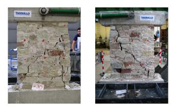
Figure 6.10: Specimen R4 at failure.
