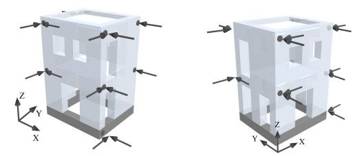
Figure 4.1: Disposition and directions of externally fixed accelerometers.
