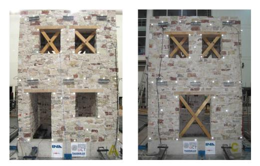
Figure A.14: SM model: timber braces inserted in the openings of the sides A (left) and B (right).
