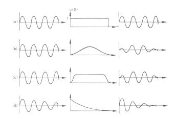
Figure 1.48: Different types of window: (a) without windowing; (b) Hanning window; (c) Cosine Taper; (d) Exponential window [Ewins, 1984].
