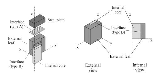
Figure 7.3: Outline of the multi-material model (left); external and internal view of the specimen (right).
