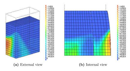
Figure 7.7: Tensile stresses in the horizontal X direction at 4.72N/mm<sup>2</sup>, model R2.
