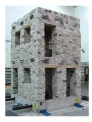
Figure A.11: RM model: detail of a crack occurred to a door jamb (left) and general view at the end of the test (right).
