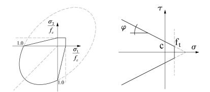
Figure 7.2: Failure criteria for solid elements (left) and interface elements (right).
