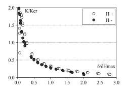
Figure 6.39: R2: Stiffness degradation.
