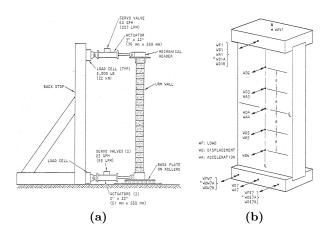
Figure 1.29: Experimental set-up (left) and sensor location (right) [ABK, 1981].
