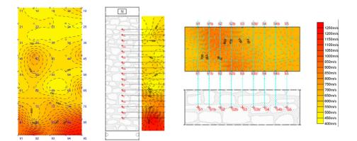
Figure 3.6: Position 1, before injection: direct sonic test (left); vertical (centre) and horizontal (right) sonic tomographies.
