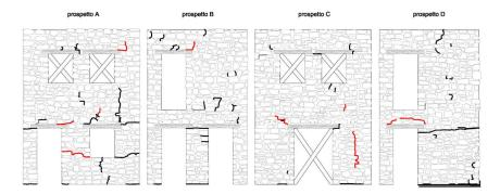
Figure 4.15: SM, crack pattern after step 0.55g in the X direction.
