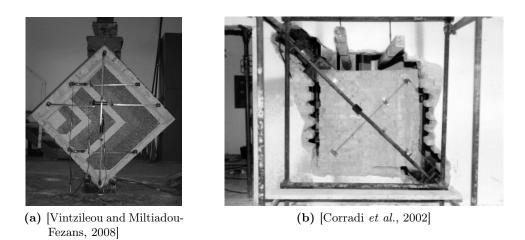
Figure 1.17: Examples of laboratory (left) and in-situ (right) diagonal compression tests.
