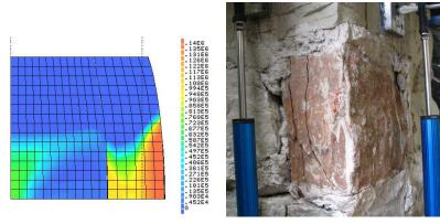
(a) Tensile stress along X, model R2(b) Experimental behaviour
