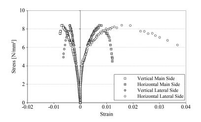
Figure 5.12: Stress-Strain behaviour on main and lateral sides of specimen R7.
