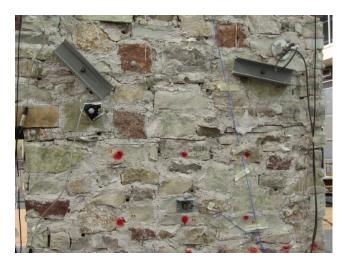
Figure A.15: SM model: horizontal crack occurred on a masonry pier.
