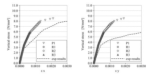
Figure 7.5: Stress-strain relationships on the horizontal directions.
