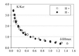
Figure 6.29: S5: Stiffness degradation.
