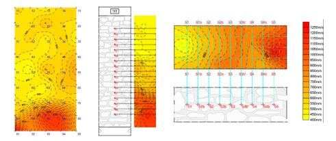
Figure 3.7: Position 2, before injection: direct sonic test (left); vertical (centre) and horizontal (right) sonic tomographies.
