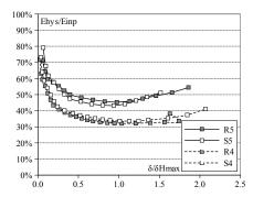
Figure 6.57: Comparison of Energy dissip- Figure 6.58: Trend of Energy dissipation<br/>ation of all specimens.for slender specimens.
