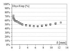
Figure 6.51: R5: Dissipated/Input Energy ratio vs displacement.
