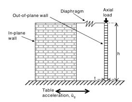
Figure 1.32: Test set-up [Simsir et al., 2004].
