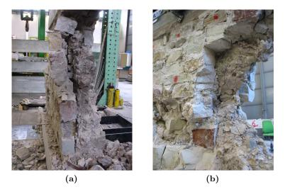
Figure 6.6: Separation of outer layers on specimens R2 (left) and S2 (right).
