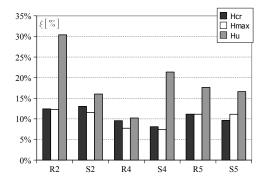
Figure 6.43: Energy ratio for all specimens at different limit states.
