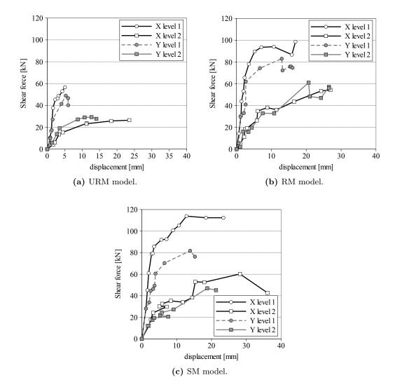
Figure 4.41: Relationships between Shear forces and corresponding storey drifts per each model.
