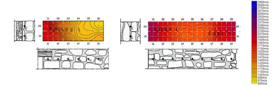
Figure 3.13: SM model: sonic tomographies before injection. Position A (left), B (right).
