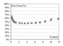
Figure 6.55: R2: Dissipated/Input Energy ratio vs displacement.
