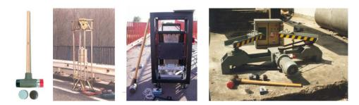
Figure 1.44: From left to right: Impulse hammer; Impulse excitation device for bridges; Electrodynamic shaker over three load cells; Eccentric mass vibrator [Cunha and Caetano, 2005].
