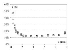
Figure 6.50: S2: Viscous damping vs displacement.
