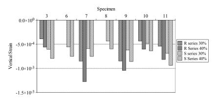
Figure 5.23: Vertical deformations for "R" and "S" series at 30% and 40% of compressive strength.
