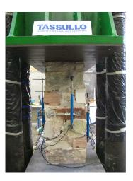
Figure 2.20: Compression experiment: test rig (left) and equipped specimen (right).
