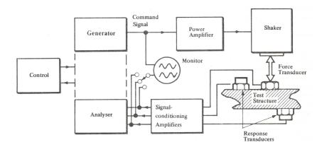
Figure 1.43: Basic components for experimental dynamic identification [Ewins, 1984].
