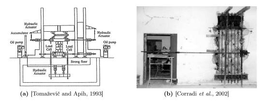
Figure 1.19: Examples of laboratory (left) and in-situ (right) shear compression tests.
