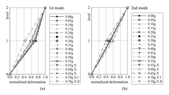
Figure 4.29: SM, first (left) and second (right) mode shape.
