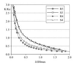
Figure 6.41: Trend of stiffness degradation for slender specimens.
