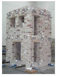
Figure 4.4: Disposition of markers to monitor the displacements.
