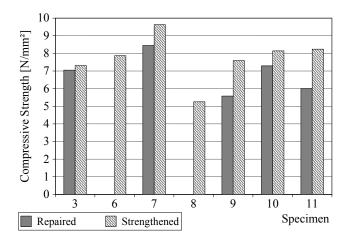
Figure 5.15: Comparison of compressive strength between specimens in the same positions.
