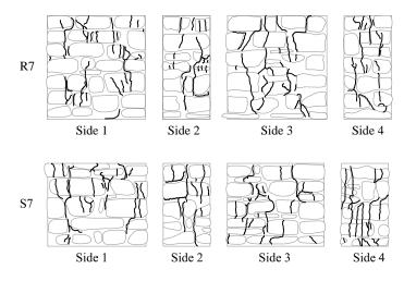
Figure 5.19: Crack pattern for R7 and S7 specimens at failure.
