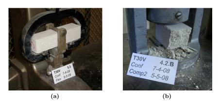
Figure 3.1: Flexural and compressive tests on mortar specimens.
