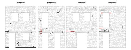
Figure 4.12: RM, crack pattern after step 0.45g.
