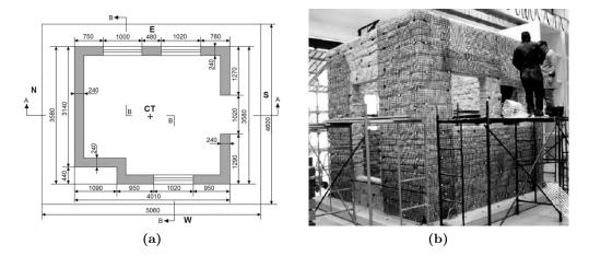
**Figure 1.39:** Floor plan of model tested by Juhásová *et al.* [2008] and strengthening intervention.
