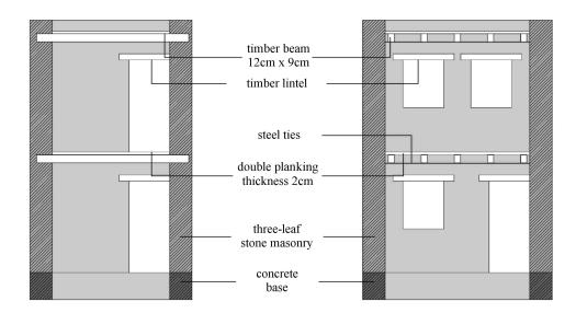
Figure 2.2: Orthogonal sections of models.
