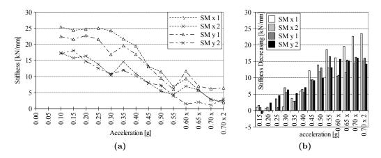
Figure 4.39: SM, Stiffness trend at increasing seismic intensity.
