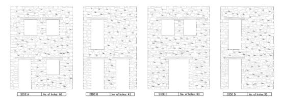
Figure 2.5: Scheme of holes executed to realize the injection.
