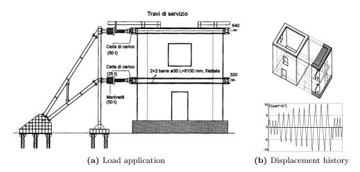
Figure 1.21: Experimental set-up designed by Beolchini et al. [1997a].
