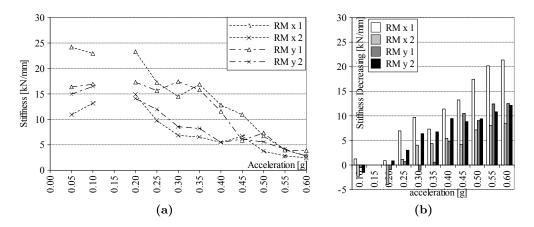
Figure 4.38: RM, Stiffness trend at increasing seismic intensity.
