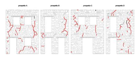
Figure 4.10: URM, Crack pattern after step 0.25g.
