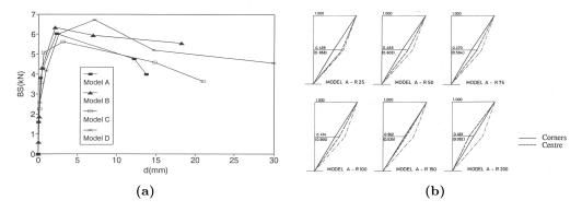
Figure 1.36: Analysis of Base Shear (left) and mode shapes (right) [Tomaževič et al., 1992].
