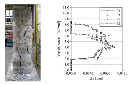
Figure 7.6: Gap between External leaf and Internal core: experiment (left) and FE model (right).
