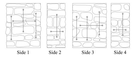
Figure 5.2: Example of instrumentation for squat specimens; type "B".
