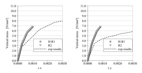
Figure 7.17: Stress-strain relationships on the horizontal directions.
