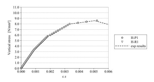
Figure 7.12: Stress-strain relationships on the vertical direction.
