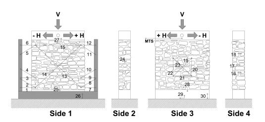
Figure 6.2: Instrumentation of a specimen and load application.
