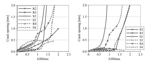
**Figure 6.28:** Lateral crack opening as a function of  $\delta/\delta_{H,max}$  of both sides.
