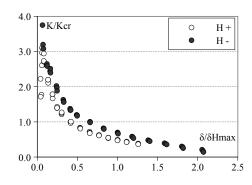
Figure 6.35: R5: Stiffness degradation.
