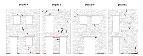
Figure 4.14: SM, crack pattern after step 0.45g.
