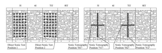
Figure 3.5: Position of sonic grids on masonry panels: direct tests (left) and tomographies (right).
