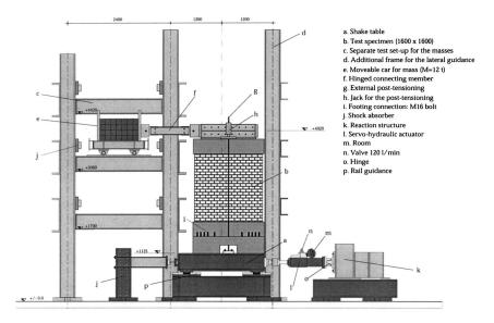
Figure 1.28: Set-up of dynamic tests employed by ElGawady et al. [2005].
