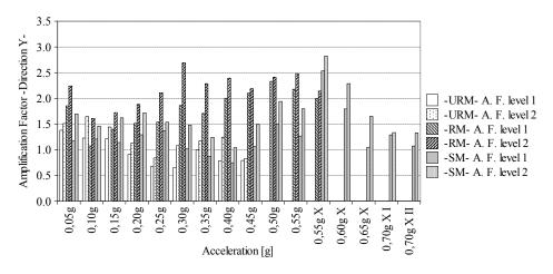
Figure 4.21: Comparison of Amplification Factors of Models, Y direction.
