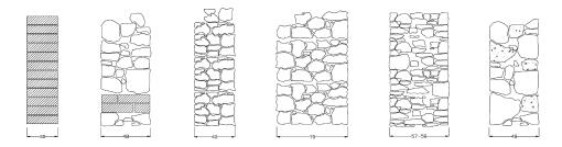
Figure 1.25: Survey of the thickness of testes masonry panels [Corradi et al., 2003].
