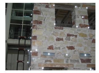
Figure A.3: URM model: detail of the damage at 0.45g.
