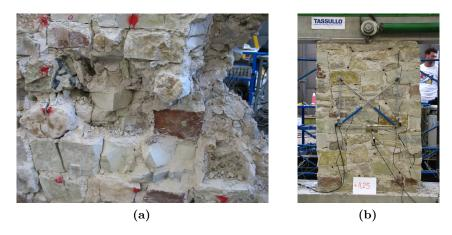
Figure 6.4: Cracks occurring in stones (left) and the formation of sub-vertical cracks (right) on specimen R5.
