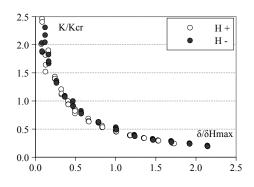
Figure 6.33: S2: Stiffness degradation.
