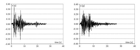
Figure 4.8: Processing of the the Montenegro earthquake on X (left) and Y (right) directions, considering the scale factor of 2:3.
