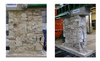
Figure 6.19: Specimen S4 at failure.
