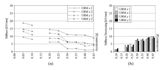
Figure 4.37: URM, Stiffness trend at increasing seismic intensity.
