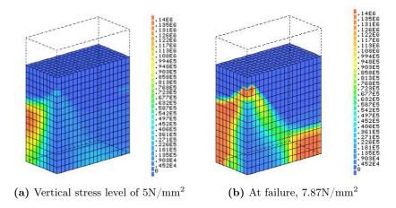
Figure 7.14: Distribution of tensile stress in the horizontal X direction, model H-R1.
