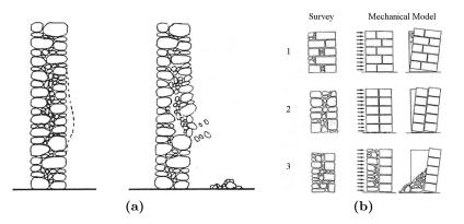
Figure 1.7: Out-of-plane failure (left) and simplified models (right) for multi-leaf stone masonry walls [Giuffrè *et al.*, 1993].
