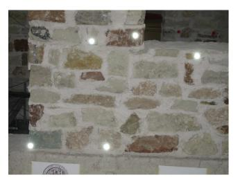
Figure A.5: URM model: detail of the damage at 0.45g.
