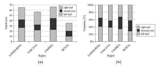
Figure 1.6: Typical depth of each leaf (left) and percentage on the overall cross thickness (right).
