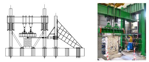
Figure 2.21: Cyclic shear compression test set-up and rig: drawing (left) and view (right)
