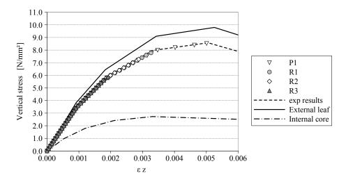
Figure 7.4: Stress-strain relationships on the vertical direction.
