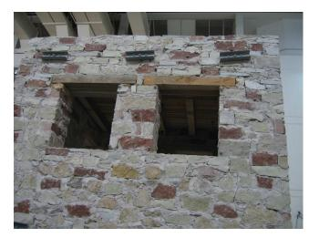
Figure A.6: URM model: detail of the damage at 0.45g.
