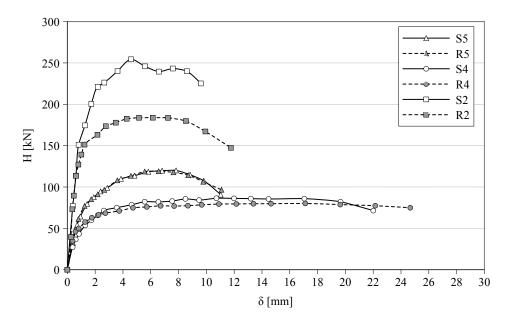
Figure 6.25: Envelopes of hysteresis loops for all the tested specimens.
