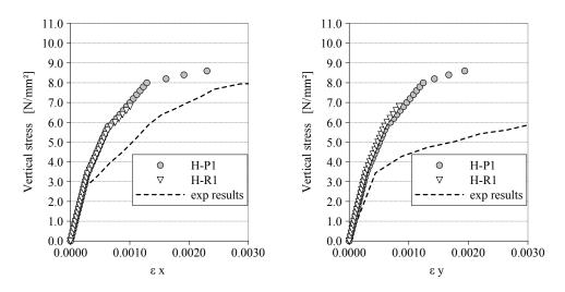
Figure 7.13: Stress-strain relationships on the horizontal directions.
