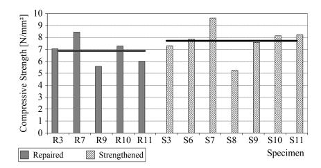
Figure 5.14: Compressive strength for the "R and "S" series.
