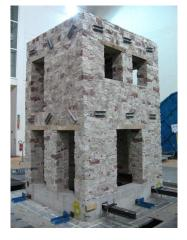
Figure A.12: RM model: two different general views at the end of the test.
