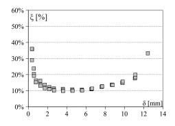
Figure 6.52: R5: Viscous damping vs displacement.
