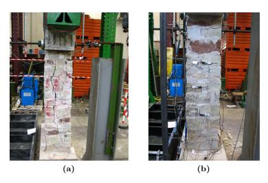
Figure 6.5: Examples of lateral cracks for specimens S5 (left) and R5 (right).
