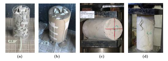
Figure 3.4: Preparation of specimen: (a) and (b); determination of indirect tensile (c) and compressive strength (d).
