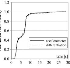
Figure 4.34: Comparison between recorded accelerations and those computed starting from displacements.
