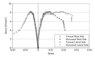
Figure 5.13: Stress-Strain behaviour on main and lateral sides of specimen S11.
