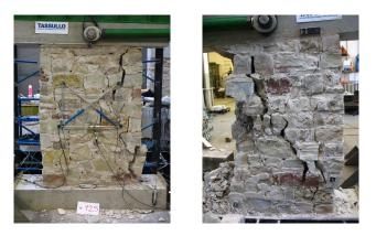
Figure 6.13: Specimen R5 at failure.
