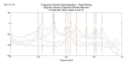
Figure 1.52: plot of the singular values of the spectral density matrices by the FDD method [Cunha and Caetano, 2005].
