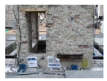
Figure A.7: RM model: steel profile to block a masonry pier.
