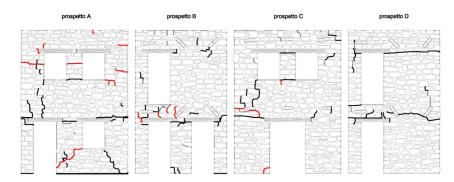
Figure 4.13: RM, crack pattern after step 0.60g, end of experiment.
