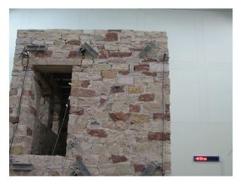
Figure A.2: URM model: detail of the damage at 0.45g.
