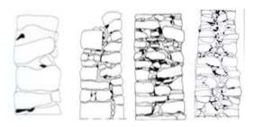
Figure 1.4: Classification of different cross sections of stone masonry: single-leaf, double-leaf without and with interlocking, three leaves [Binda, 1999].
