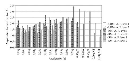
Figure 4.20: Comparison of Amplification Factors of Models, X direction.
