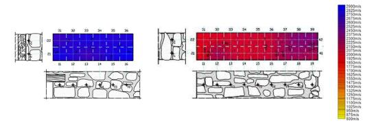
Figure 3.16: SM model: sonic tomographies after injection. Position A (left), B (right).
