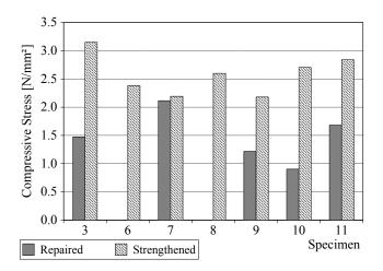
Figure 5.4: First crack appearance: comparison of compressive stress between specimens in the same position.
