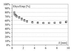
Figure 6.49: S2: Dissipated/Input Energy ratio vs displacement.
