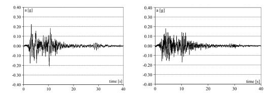
Figure 4.7: Time history of Montenegro earthquake on X (left) and Y (right) directions.
