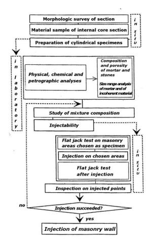
Figure B.1: Description of the followed procedure to study the injectability of a masonry (Binda et al., 1998)
