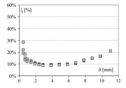
Figure 6.46: S5: Viscous damping vs displacement.
