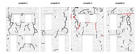
Figure 4.11: URM, crack pattern after step 0.45g, end of experiment.
