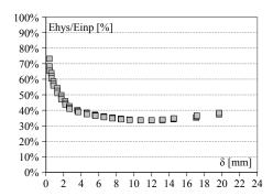
Figure 6.47: S4: Dissipated/Input Energy ratio vs displacement.
