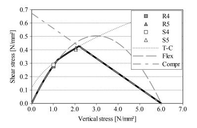
Figure 6.64: Failure field of tested slender specimens.
