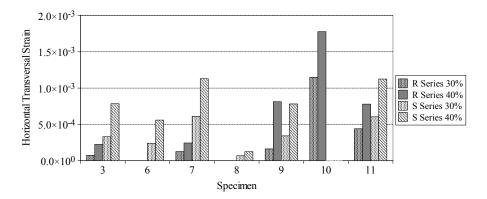
Figure 5.22: Horizontal deformations for the "R" and "S" series at 30% and 40% of compressive strength.
