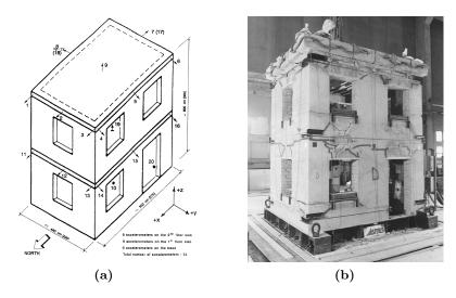
Figure 1.37: Design (left) and test (right) of the building model [Benedetti et al., 1998].
