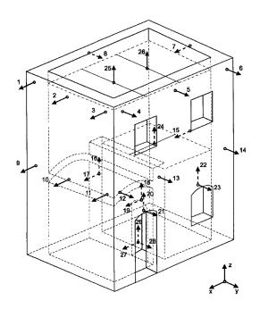
Figure 1.41: Axonometric view of tested building specimen [Juhásová et al., 2002].
