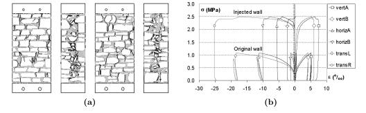
Figure 1.14: Examples of specimen and stress-strain relationship [Valluzzi, 2000].
