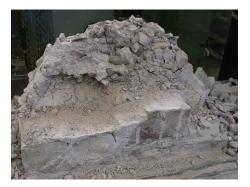
Figure 5.11: Destroyed core of specimen S11 after the test.
