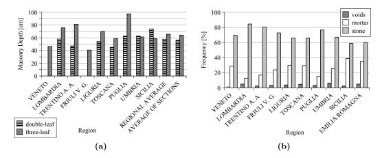
Figure 1.5: Percentage of materials on typical cross sections (left) and kind of transversal typology (right).
