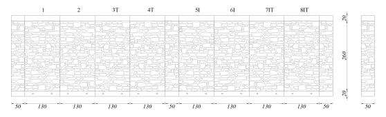
Figure 2.10: Design of panels with relative acronym.
