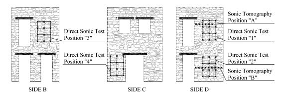
Figure 3.9: Position of sonic grids on masonry buildings: direct tests and tomographies.
