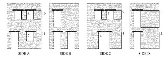
Figure 2.19: Scheme of position from where specimens for quasi-static tests were obtained.
