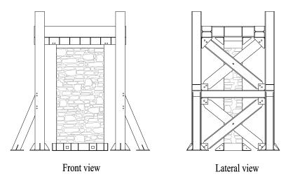
Figure 2.18: Design of the steel frame: front (left) and lateral (right) view.
