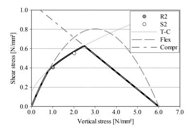
Figure 6.63: Failure field of tested squat specimens.
