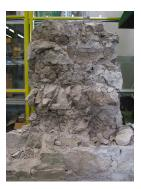
Figure 5.8: Front view of specimen R7 after the test.
