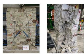
Figure 6.22: Specimen S5 at failure.
