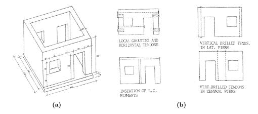
Figure 1.34: Geometry of models and examples of strengthening interventions [Benedetti, 1980].
