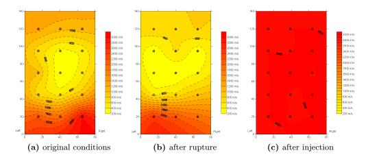
Figure B.2: Application of sonic tomography to a multi-leaf stone masonry wall (Valluzzi, 2003).
