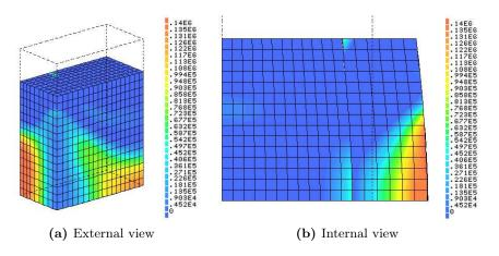
Figure 7.9: Tensile stresses in the horizontal X direction at 8.07N/mm<sup>2</sup>, model P1.
