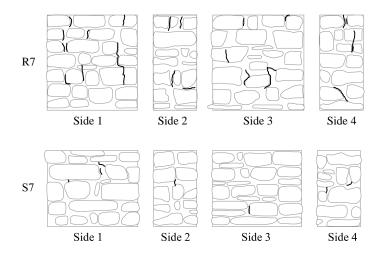
Figure 5.16: Crack pattern for R7 and S7 specimens at 4.20 N/mm<sup>2</sup>.
