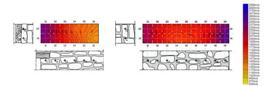
Figure 3.12: URM model: sonic tomographies before injection. Position A (left), B (right).
