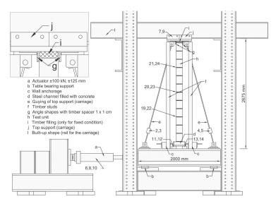
Figure 1.33: Set-up for dynamic tests with detail of the top support [Wilhelm et al., 2007].
