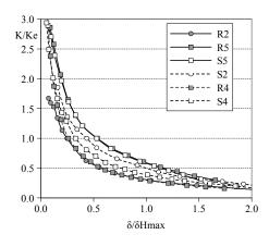
Figure 6.42: Comparison of the stiffness degradation of all specimens.
