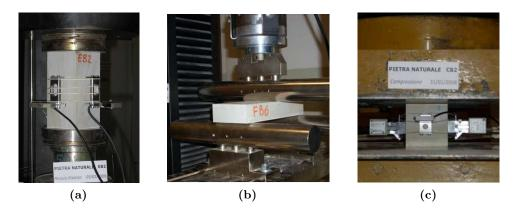
Figure 3.2: Determination of elastic modulus and of flexural and compressive strength of stone specimens.
