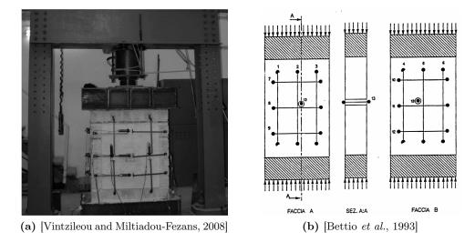
Figure 1.11: Examples of laboratory (left) and in-situ (right) compression test.
