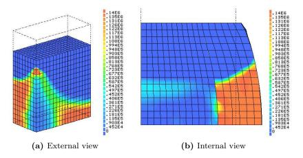
Figure 7.8: Tensile stresses in the horizontal X direction at failure, model R2.
