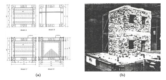
Figure 1.35: Design of different floor typologies (left) and test of a building model (right) [Tomaževič *et al.*, 1992].
