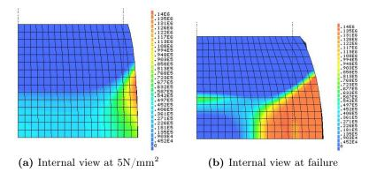
Figure 7.18: Distribution of tensile stress in the horizontal X direction, model H-R1.
