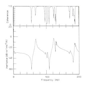
Figure 1.50: Examples of inertance and phase of a dynamic identification [Ewins, 1984].
