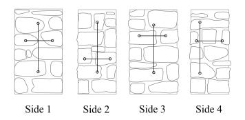
Figure 5.1: Example of instrumentation for slender specimens: type "A".
