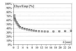
Figure 6.53: R4: Dissipated/Input Energy ratio vs displacement.
