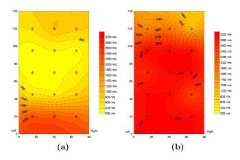
Figure 1.10: Example of comparison of sonic velocities before (left) and after (right) injection of lime grout [Valluzzi, 2000].
