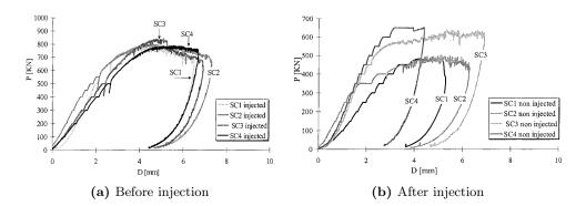
Figure 1.15: Load-vertical displacement curves of stone samples [Toumbakari, 2002].
