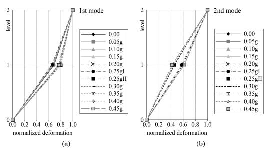
Figure 4.27: URM, first (left) and second (right) mode shape.
