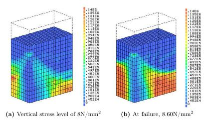
Figure 7.15: Distribution of tensile stress in the horizontal X direction, model H-P1.
