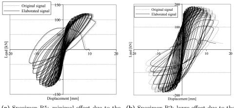
(a) Specimen R5: minimal effect due to the processing of the original signal.(b) Specimen R2: large effect due to the processing of the original signal.
