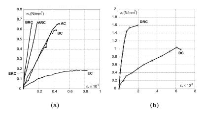
Figure 1.13: Stress-strain relationship of tested specimens [Modena, 1999].
