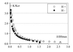
Figure 6.31: S4: Stiffness degradation.
