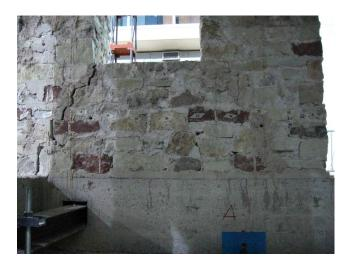
Figure A.10: RM model: a crack occurred at first floor level, internal view.
