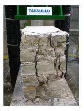
Figure 5.7: Lateral view of specimen S11 after the test.
