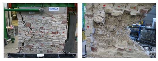
Figure 6.16: Specimen S2 at failure.
