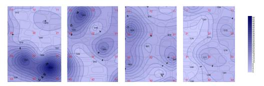
Figure 3.14: SM model: Maps of injected grout (litres). From left to right: position 1 to 4.
