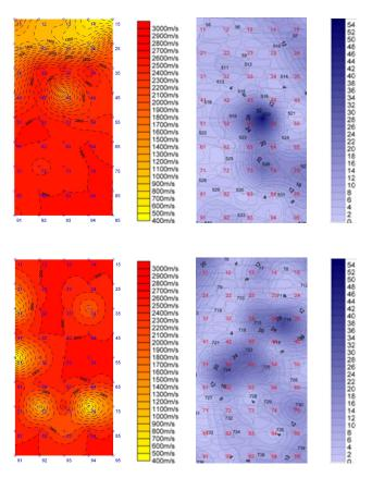
Figure 3.8: Position 1 (top) and 2 (bottom), after injection: direct sonic tests (left) and quantity of injected grout (right) in litres.
