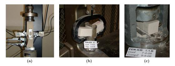
Figure 3.3: Determination of elastic modulus and of flexural and compressive strength of grout specimens.
