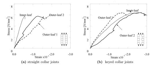
Figure 1.16: Stress-strain curve on different masonry layers [Binda et al., 2006].
