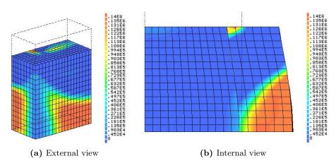
Figure 7.10: Tensile stresses in the horizontal X direction at failure, model P1.
