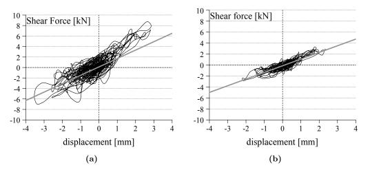
Figure 4.36: Example of hysteresis loops for SM model on the first (left) and second (right) storey in the X direction (0.40g).
