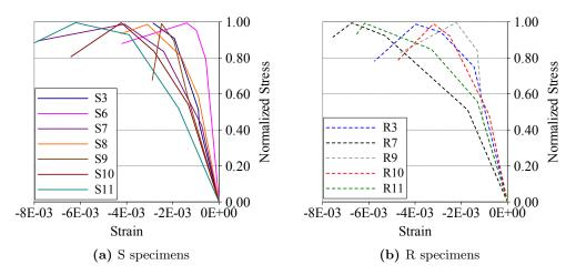
Figure 5.25: Oversimplified normalized compression behaviour of all tested specimens.
