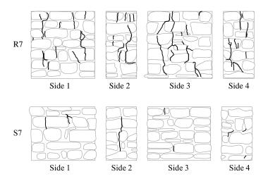
Figure 5.17: Crack pattern for R7 and S7 specimens at 7.00 N/mm<sup>2</sup>.
