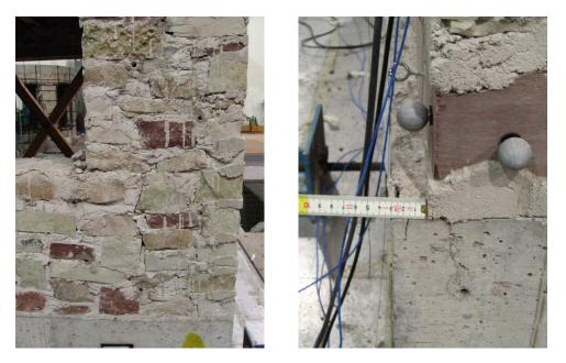
Figure A.13: SM model: detail of a crack occurred at the first floor level (right) and bottom displacement of a pier.
