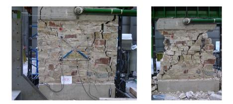
Figure 6.7: Specimen R2 at failure.
