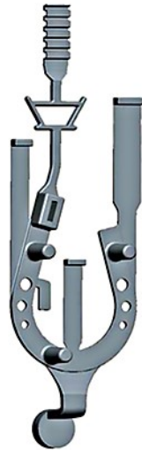
Fig. 11 Horse-shoe reference casting
