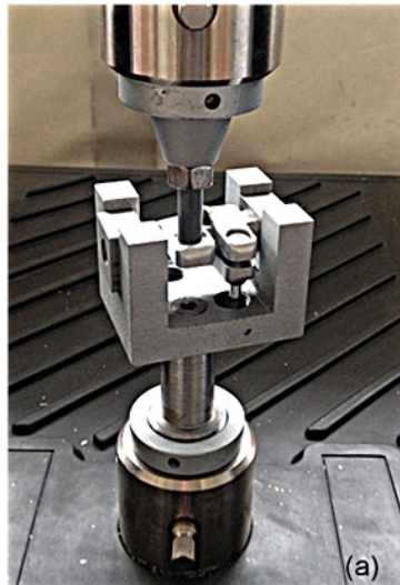
Fig. 19 Ongoing mechanical test carried out on the sleeve casting
