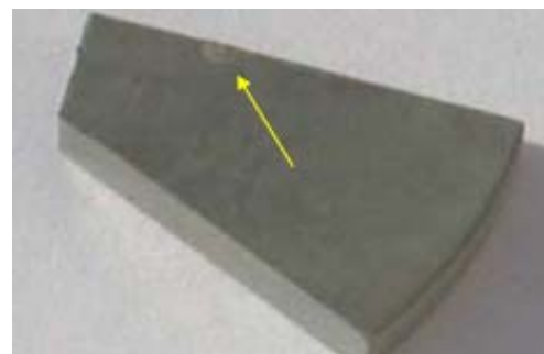
Figure 5.16- Local defect in the oxide scale on an Cr - coated sample after 500 h of oxidation at 1000 °C
