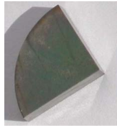
Figure 5.6 - Cr - coated sample appearance after interdiffusion treatment
