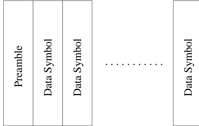
Figure 2.6: Basic frame structure.
