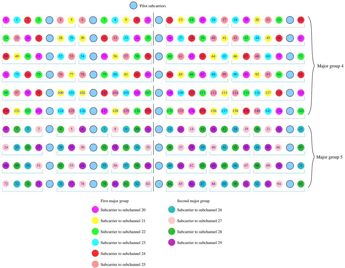
Figure 7.13: Subcarrier allocation into subchannels, for the last two major group, considering a DL\_PermBase equal to 15.
