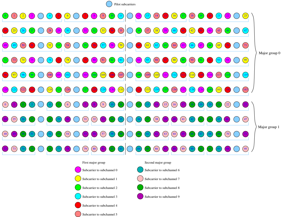
Figure 7.12: Subcarrier allocation into subchannels, for the first two major group, considering a DL\_PermBase equal to 0.
