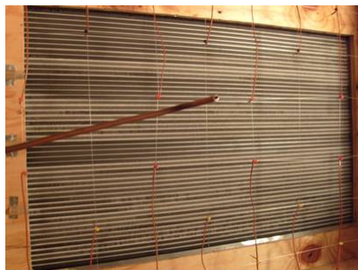
Figure 1.7.15(b): MCHX evaporator (with IHX) after 2500 sec
