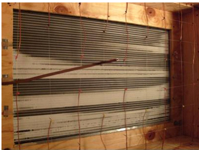
Figure 1.7.14(a): MCHX evaporator after 1800 sec
