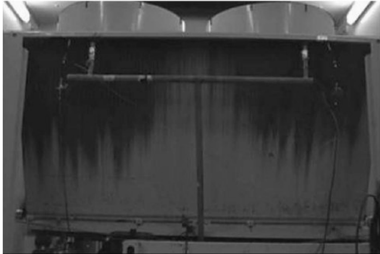
Figure 1.5.38: The microchannel evaporator at the end of the frosting cycle; (Shao et al. , 2009)
