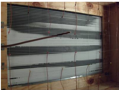
Figure 1.7.15(a): MCHX evaporator after 2500 sec
