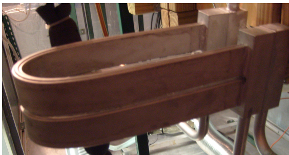
Figure 1.7.7: The internal heat exchanger (IHx).
