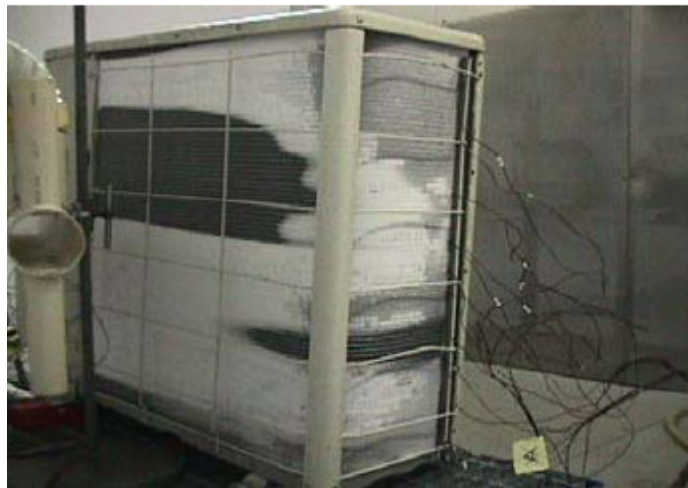
Figure 1.5.7: Frosting of a 3-passage microchannel evaporator (Macri, 2006)
