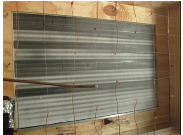
Figure 1.7.10: The round tube evaporator at the end of a frosting cycle
