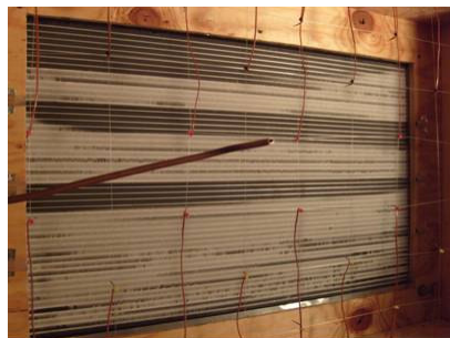
Figure 1.7.16(b): MCHX evaporator (with IHX) after 3600 sec
