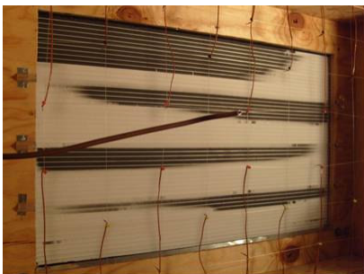
Figure 1.7.16(a): MCHX evaporator after 3600 sec
