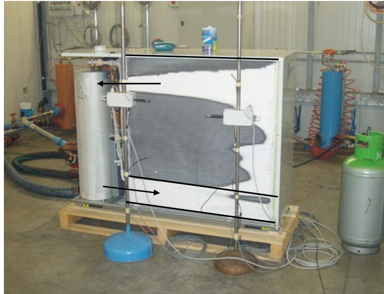
Figure 1.5.6: Frosting of a 2-passage microchannel evaporator
