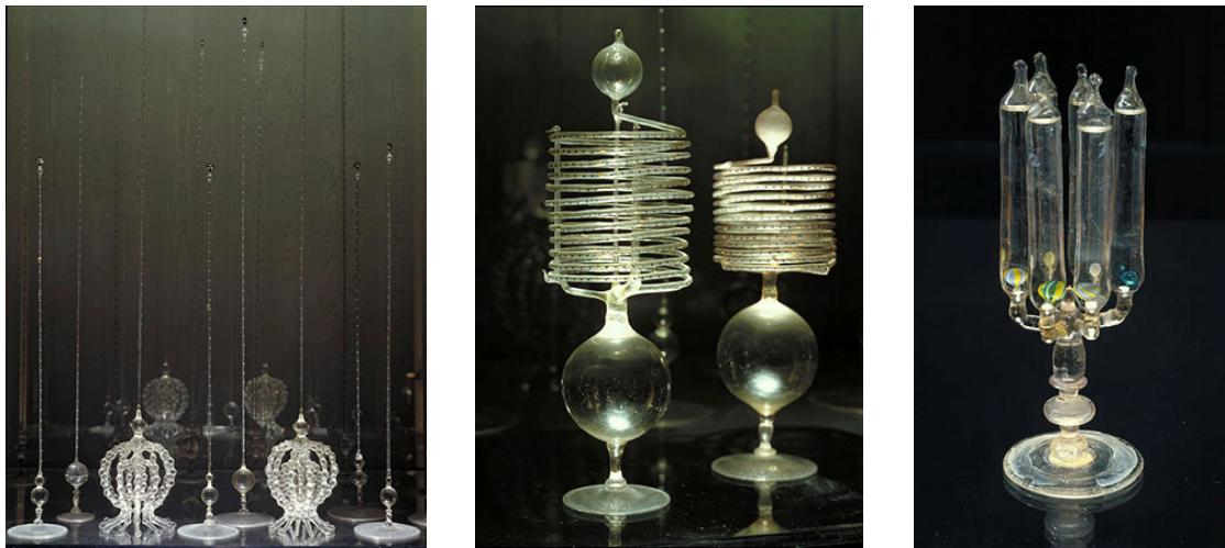
Figure 4.6: From the left to the right: a) Tall-stem thermometer: The stem carries enamel buttons indicating the degrees of one of the thermometric scales used by the Accademia del Cimento (1657-1667). The black buttons indicate single degrees, the white buttons 10 degrees, and the blue buttons 100 degrees. b) Spiral thermometer: thermometer with spiral or "snail" stems used by the Accademia del Cimento. 420 enamel buttons indicate the degrees: the black buttons indicate single degrees, the white buttons 10 degrees, and the blue buttons 100 degrees. c) Cluster thermometer called "infingardo" (slothful): this thermometer used by the Accademia del Cimento consisted of six phials, numbered from 1 to 6, clustered on a column. The phials contain alcohol, in which small glass spheres of different density are immersed.
