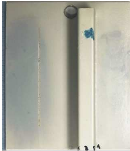
Figure 10.7: Demonstrator (AA6013 and AA6061) produced at EADS Deutschland GmbH after 1000h alternate immersion emersion test according to DIN EN 3212.
