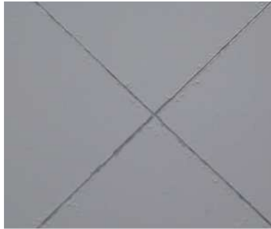
Figure 10.11: Demonstrator (AA3105) produced at Plalam SpA after salt spray test
