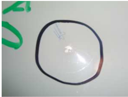
Figure 10.9: Demonstrator (AA7075) produced at Hellenic Aerospace Industry S.A. after impact resistance test according to ISO 6272
