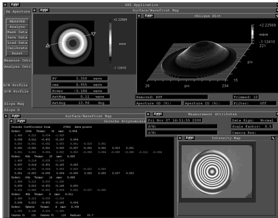
Figure 28: Interferogram for a single lens. The wave surface after a double passage through the lens (as in configuration depicted in Figure 27) is analyzed. On the right the shape of the wavefront is reproduced above the interference pattern. On the left the interferometer software returns the Zernike polynomial expansion describing the wavefront.
