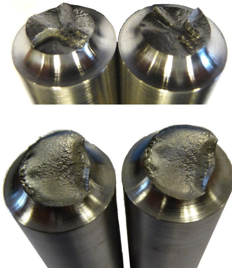
Figure 6.6.2. Typical fracture surface from a semicircular notch under multiaxial loading: in phase (a) and out-of-phase (b)
