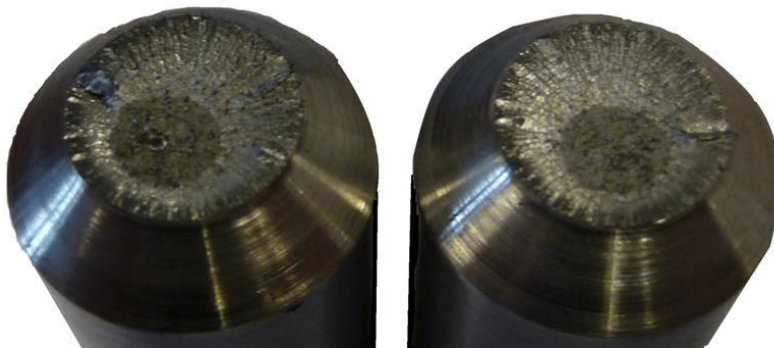
Figure 6.5.3. Fracture surfaces from V-notched specimens under multi-axial fatigue: \lambda=0.6 and \Phi=0^\circ
