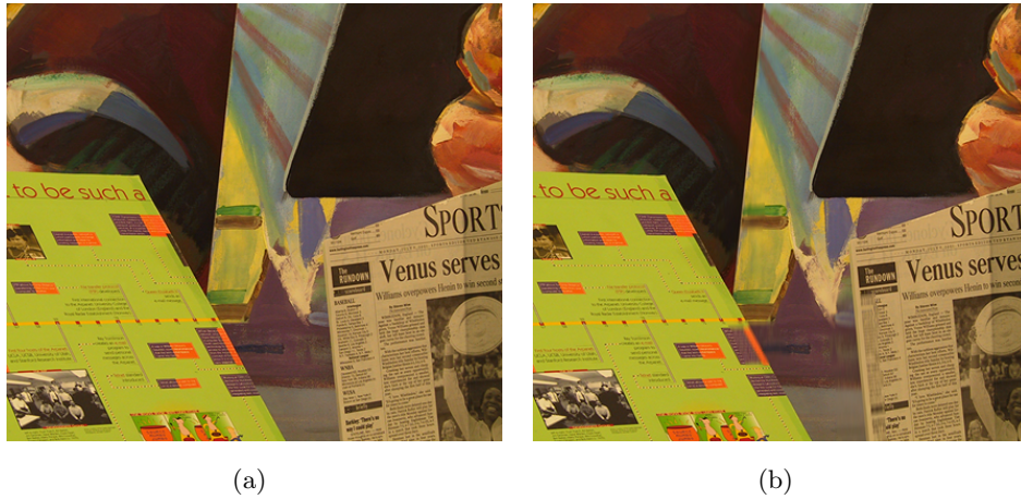
Figure 3.5: Results of directional filtering: (a) Reference image, (b) Reference image after the application of the directional Gaussian filter.
