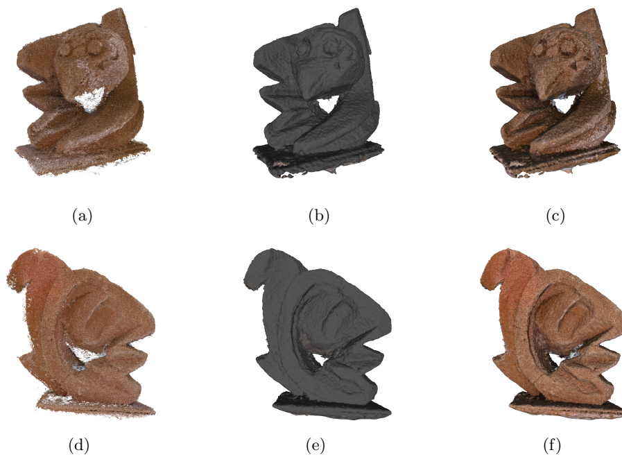
Figure 6.10: 3D reconstruction of the Civetta dataset, (a) Pointcloud, front view, (b) Mesh, front view, (c) Textured mesh, front view, (d) Pointcloud, back view, (e) Mesh, back view, (f) Textured mesh, back view.
