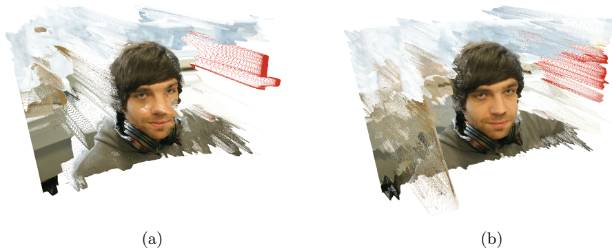
Figure 6.6: Results comparison in two view 3D reconstruction based on the combination of CoMEDE and University of Dortmund OF, (a) SAD matching criteria, (b) BCC matching criteria.
