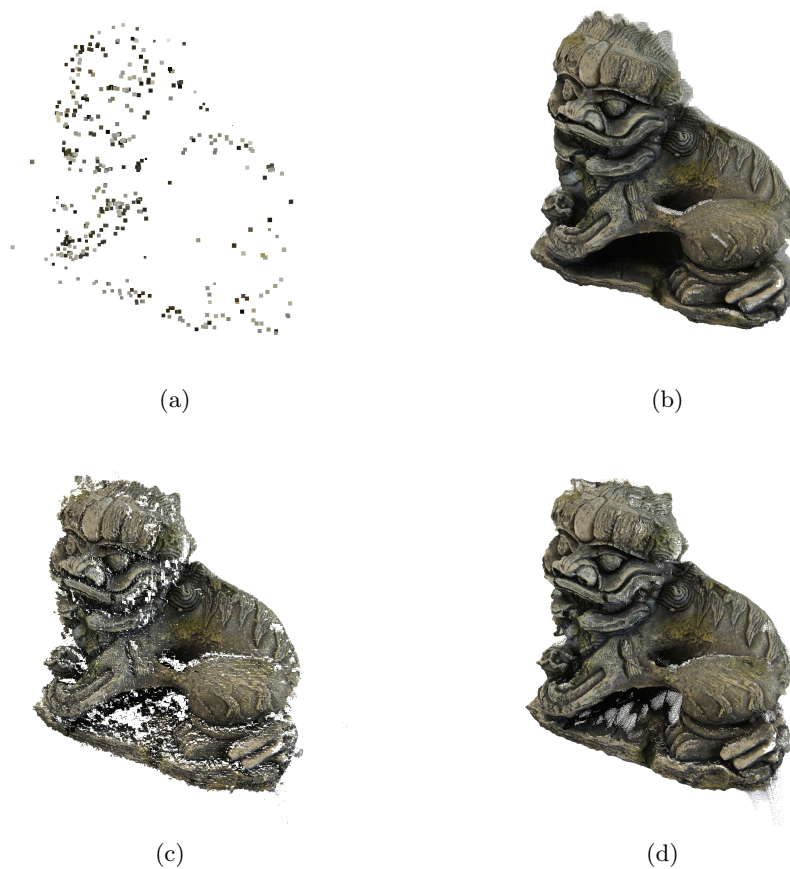
Figure 6.5: Results comparison in two view 3D reconstruction, (a) Features based 3D reconstruction, (b) University of Dortmund OF based 3D reconstruction, (c) CoMEDE based 3D reconstruction, (d) combination of CoMEDE and University of Dortmund OF based 3D reconstruction.
