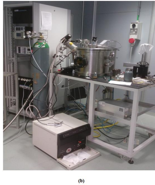
Figure A.3a) The basic principle of the sputtering deposition technique, b) Typical diagram of the Magnetron sputtering facility located at CNR-Padova, Italy.
