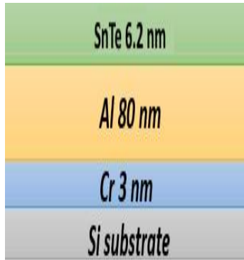
Figure 5.2. The nominal structure of the sample as monitored with a quartz microbalance during the deposition.
