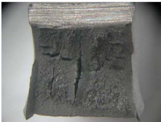
Fig. 8. Fracture surface of the 2101 steel aged at 650 °C for 45 min.
