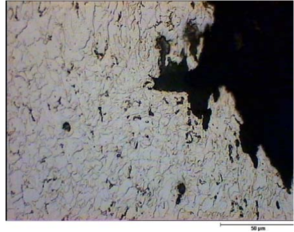
Fig. 4. Transgranular fracture with microvoids and local plastic deformation.
