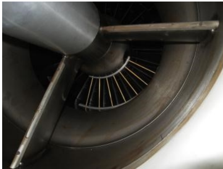
Figure A9 Partial inlet distortion grid installed at the compressor inlet.
