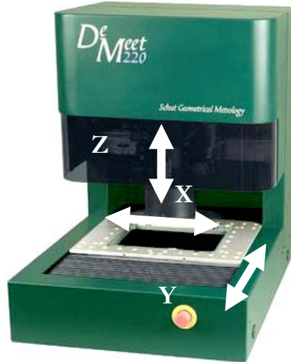
Figure 6.2 – DeMeet 220 camera and table movements
