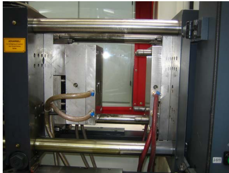
Figure 5.2 – The Ferromatik Milacron K 60 injection molding machine at the IPL/DTU Polymer Centre. Mold and clamping system.
