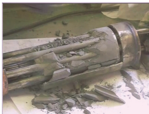
Figure 5.1 \text{Mg}/\text{MgH}_2 powder compaction during cycling experienced in the reactor studied in ref. [5.11].
