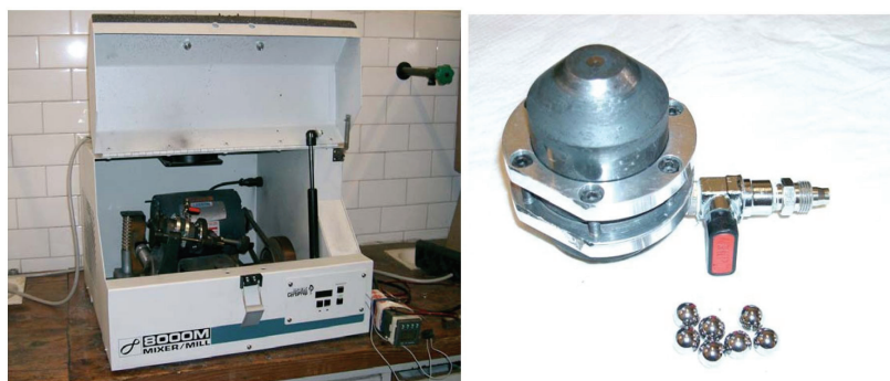
Figure 3.1 SPEX 8000M shaker mill (left) and home made vial with stainless steel balls (right).
