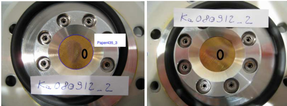
Figure 4.17: An example of the "virgin" area (left) and "beamspot" area (right) measured position for the target Ka2. The beam position is defined by the black circle. This circle has been superimposed on the target picture by a graphic software.
