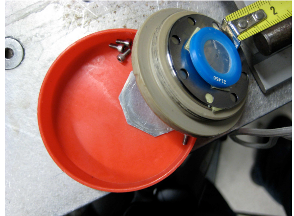
Figure 4.29: Pos 1 for the source during the efficiency measurements. The position scheme is shown in the left panel. The backing is represented in black, the ring in blue the source in red and the plastic cap in light brown. The photo of the source is in the right part of the picture.
