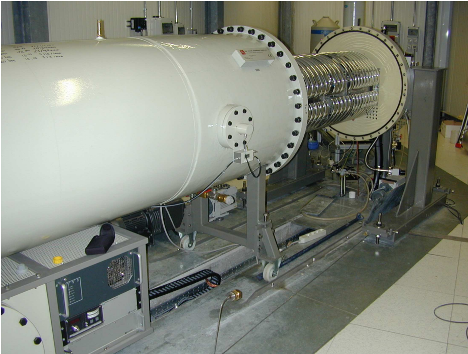
Figure 2.1: The LUNA2 400 kV accelerator with the tank open for maintenance. Inside the tank, the metallic rings, keeping the ion source free from electric fields, are visible.
