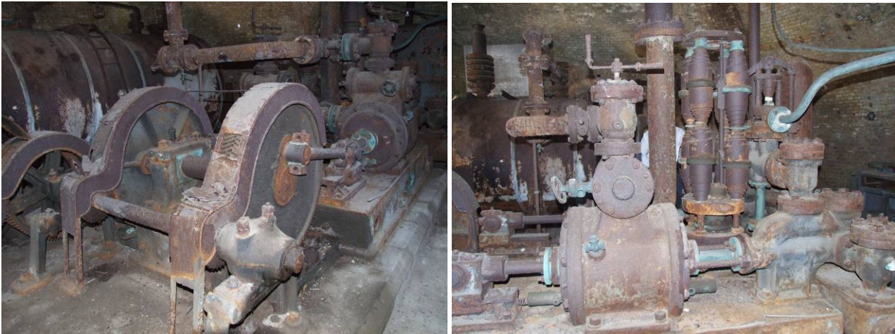
Fig. 5.3.6: The bronze parts replaced over time
