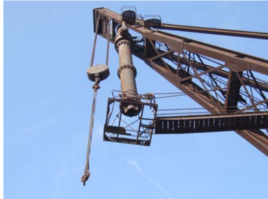
Fig. 5.6.11: Detail of the cylinder positioned in the front/upper part of the crane
