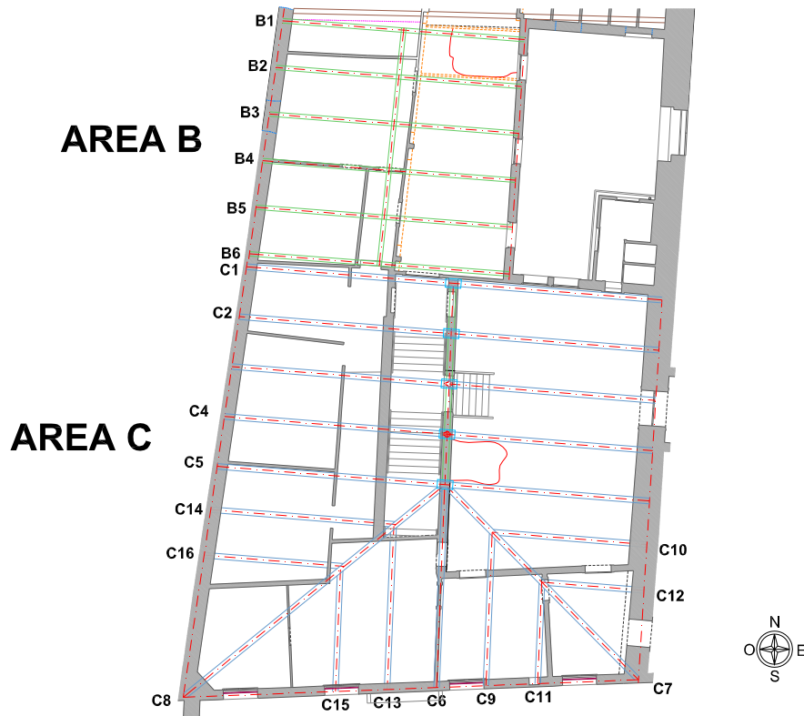
Fig. 4.4.86: Numbering of the reinforced concrete trusses
