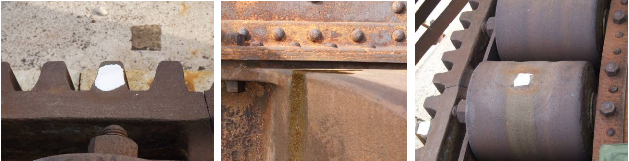
Fig. 5.4.23: Elements subjected to metallographic test (rack teeth, sliding block, roller)
