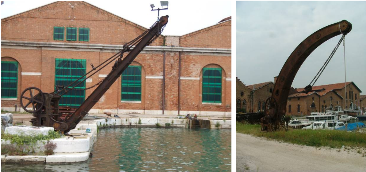
Fig. 5.2.5: The oblique boom crane in the Nappe area and the 35 tons Fairbairn gooseneck crane on the Artillery zone
