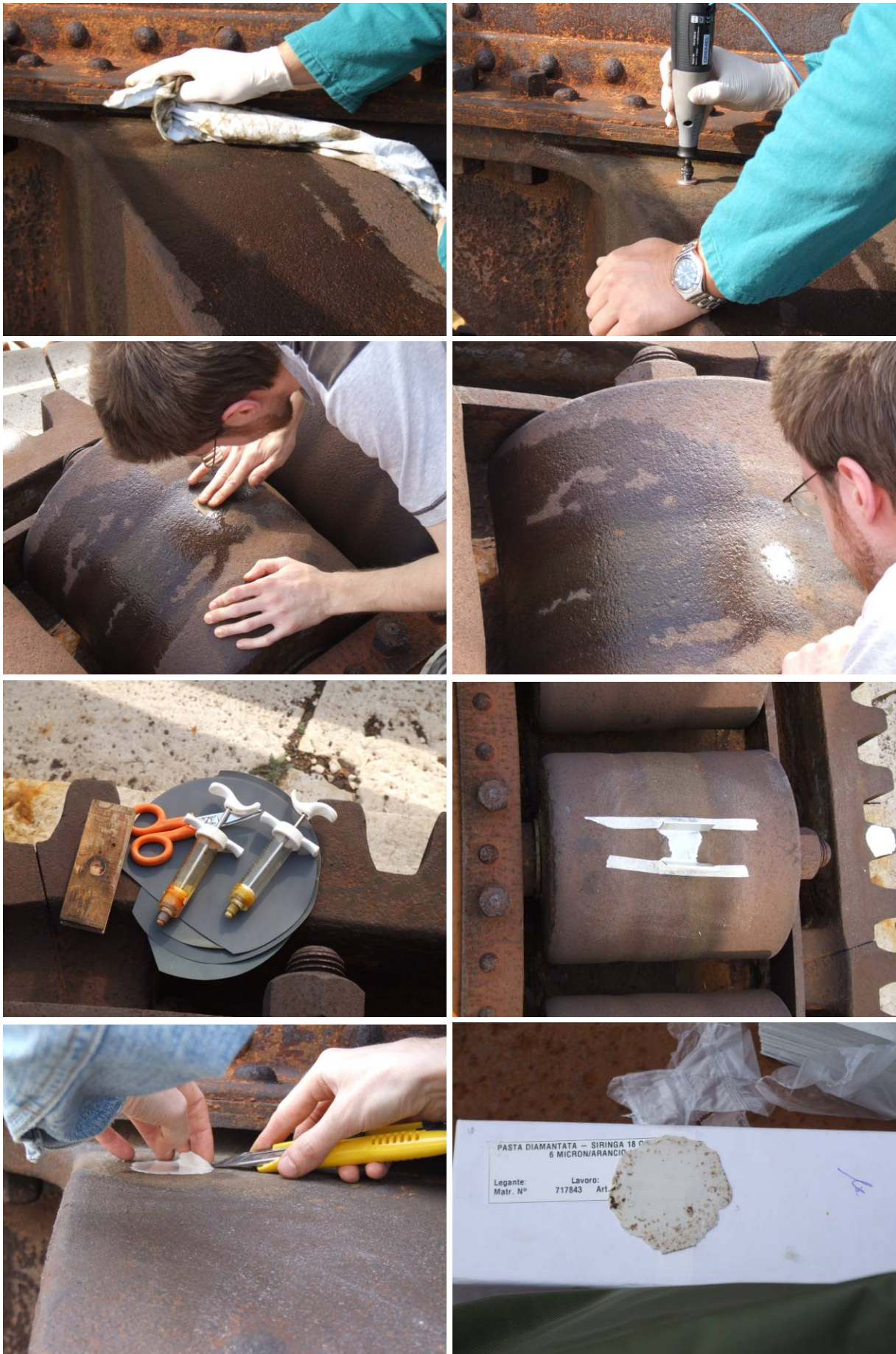
Fig. 5.4.22: Micrographs with silicon metallographic replicas
