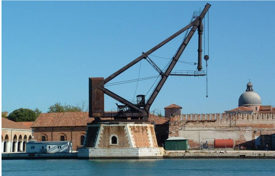
Fig. 3.10.4: The Armstrong, Mitchell & Co. hydraulic crane in the “Darsena Grande” of the Arsenale of Venice
