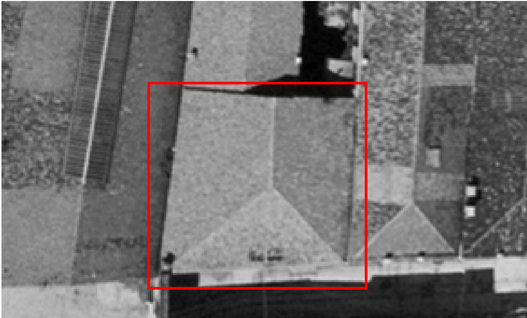
Fig. 4.4.123: Detail of the different inclination of the pitches of the area C of the Sale d'Armi Nord
