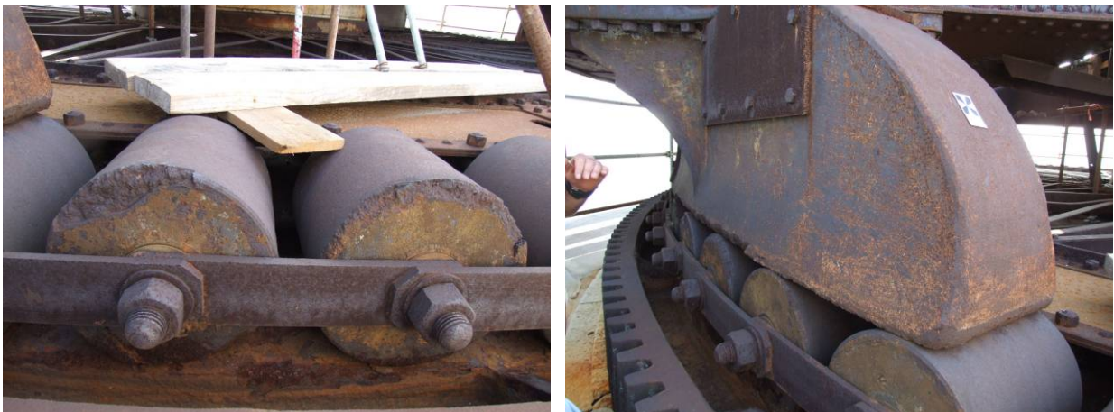
Fig. 5.4.48: Ware in rollers edges and in sliding blocks
