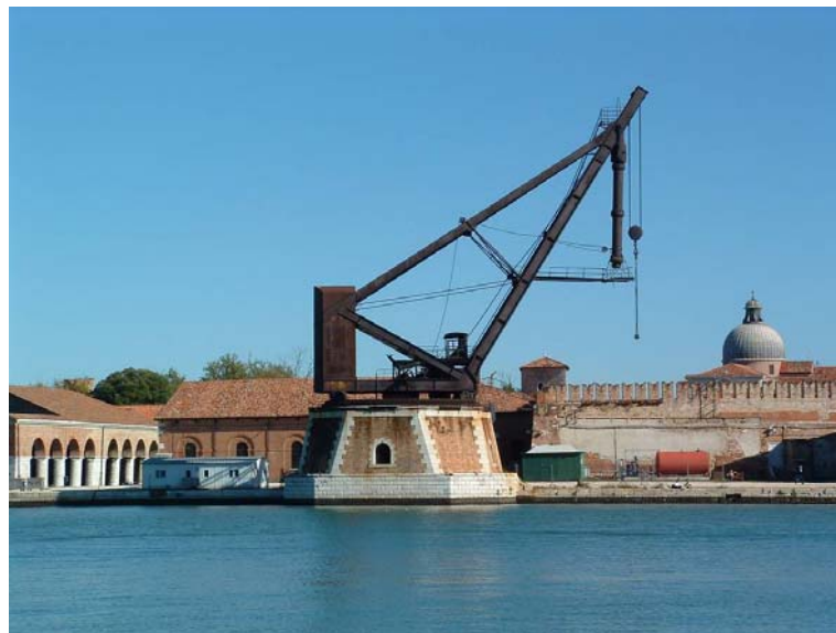
Fig. 5.2.6: The Armstrong, Mitchell & Co. hydraulic crane in the Artillery dock of the Great Basin of the Arsenal of Venice
