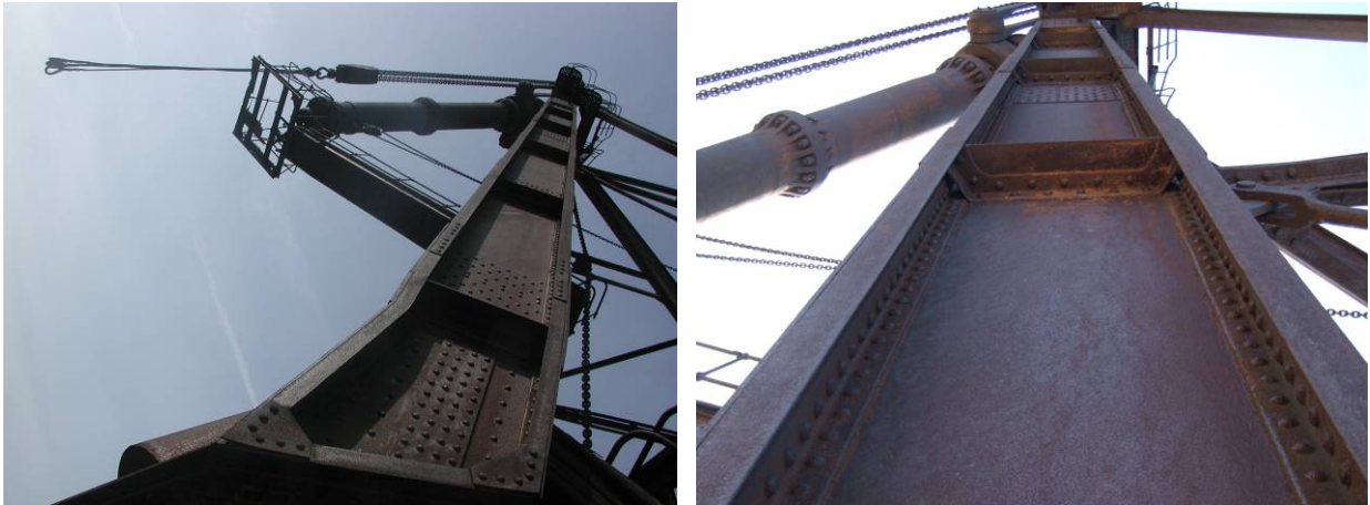
Fig. 5.3.14: The lattice boom of the crane showing its pyramid structure
