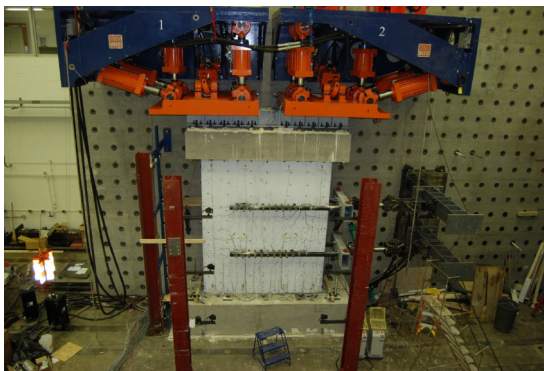
figura 2.9 – Planar Wall Test (PW1) [2.18]
