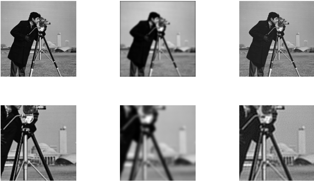
Figure 4.1.15: Upper row, from left to right: original image, blurred and noisy image, reconstructed image obtained employing Algorithm 12 and stopping at the 5-th iteration of the Arnoldi algorithm. Lower row: blow-ups of the corresponding images displayed in the upper row.
