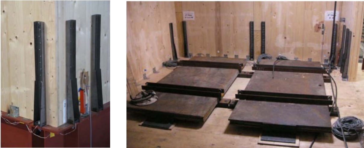
Fig. 3.4 – High-strength IVALSA hold-downs [3.21].
