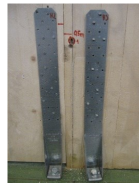
Fig. 2.5 – (a) Specimen A-1: large deformation of angle brackets, lateral yielding of hold-downs; (b) Specimen A-2: major deformation concentrated at hold-downs, and deformation of angle brackets; (c) Specimen B-1: predominant sliding and uplift of wall; (d) Specimen B-2: sliding, uplift and relative displacement of CLT plates; (e) Specimen C: pull-out of screws and nails missing due to shear failure. [2.51]
