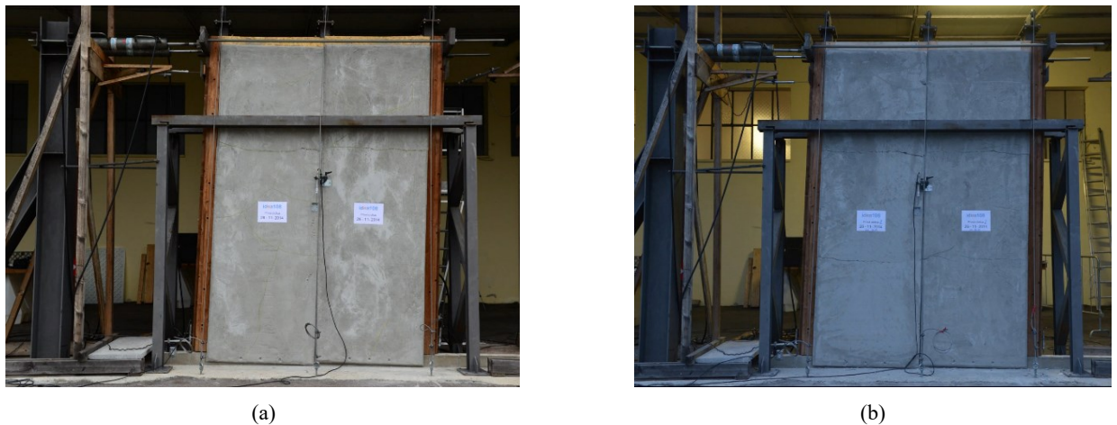
Fig. 4.17 – Wall configurations at the end of the cyclic loading tests: (a) wall A; (b) wall B.
