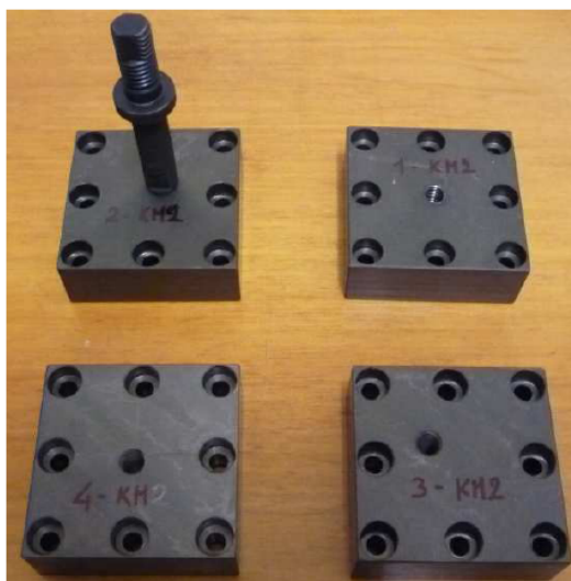
Figure 2.19: Interface plates to fix KM to a standard optical bench. They can be fixed to the bench with a maximum of 8 M6 screws, then the interface column will be inserted into the M8 threaded hole.
