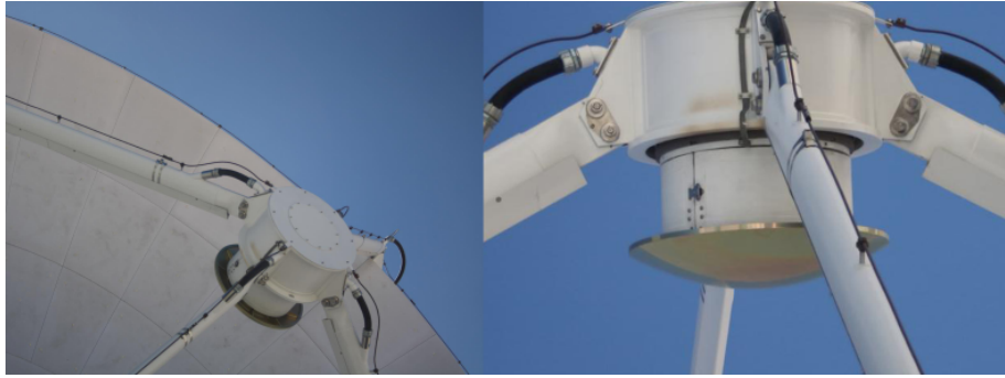
Figure 5.5: Images of the area interested by the overheating that caused the color change in the white painting of the apex structure close to the secondary mirror. The burned area is estimated to be 200-250mm large.
