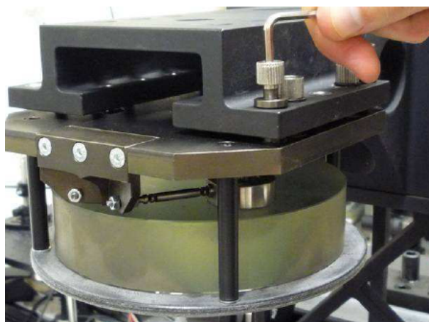
Figure 2.25: measurement of the optical path inside the KM. The distantometer is aligned with the optical axis of the KM using decenter and tip-tilt correction on the distantometer holder. Is reached an accuracy of about 200'' for tip-tilt and 0.5\text{mm} for decenter. The vertical position of M2 can be adjusted using the 3 screws over the mirror mount of M2.
