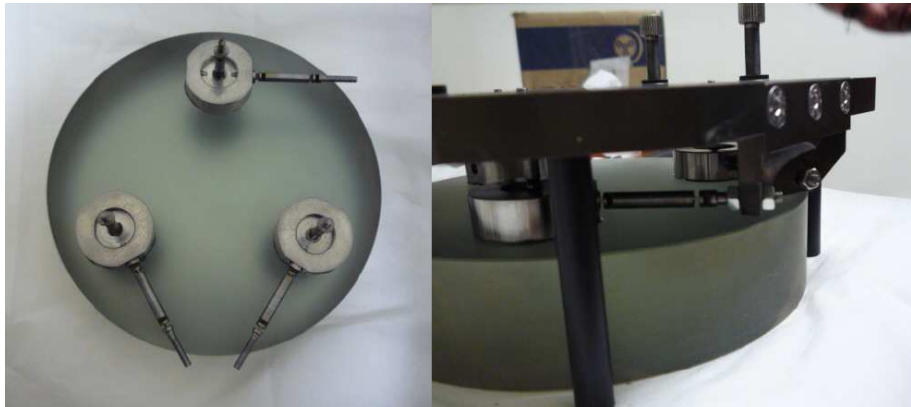
Figure 2.18: M2 unit mounting: the 6 bars are screwed on the pads. M2 with the tilting plate fixed to the horizontal bars with nuts and lock nuts, through bar supports.
