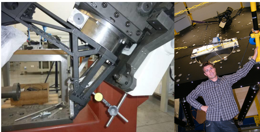
Figure 2.33: Left: a tilting bench is used to change the inclination of the system, while the flexures are measured using a mechanical comparator. Right: flexure test at the Max Planck Institute for Astronomy in Heidelberg after the internal alignment technical support. The KM SX was placed on the linc-NIRVANA bench that will be at the LBT telescope in the next future.
