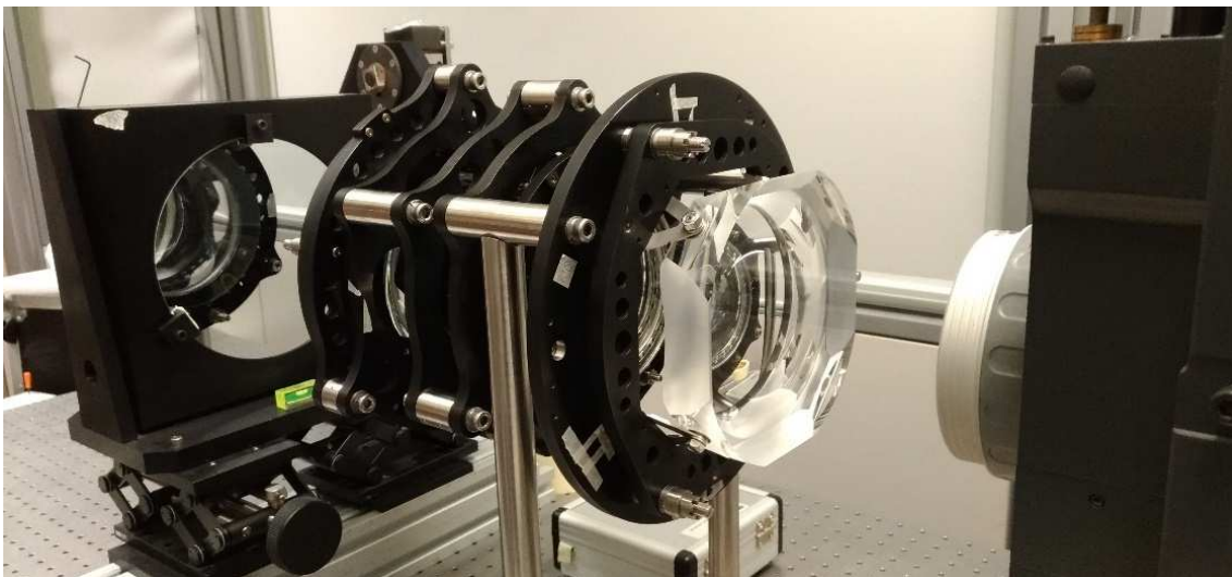
Figure 93. The double pass test to measure the accuracy of the interferometer with respect to the position and dimension of the aperture mask. Plato is illuminated in direction L6 to L1.
