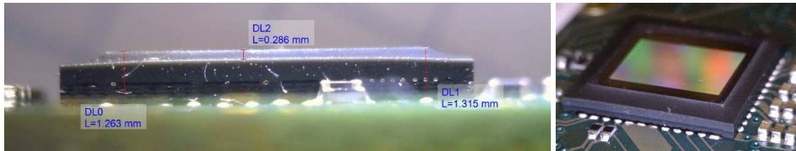
Figure 80. The optical window of the CCD, measured in thickness in the laboratory
