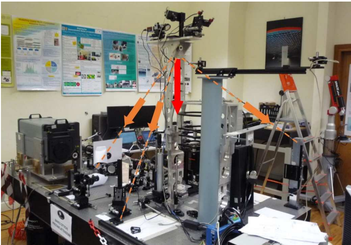
Figure 91. The three metallic ropes added to the GSE holding the prototype, with the purpose to improve the setup stability; their preload can be adjusted individually and the resulting force is directed downwards, decreasing the oscillations of the GSE tower.
