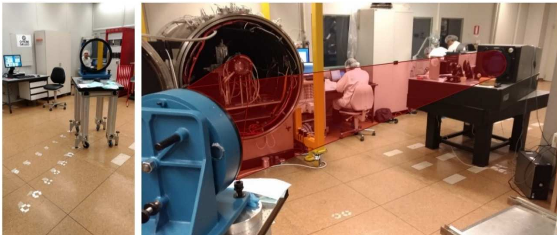
Figure 130. The TOU installed in the climate chamber. Left: the folding mirror positions for simulating the off-axis beam. Right: the large beam expander folded by the mirror inside the climate chamber.
