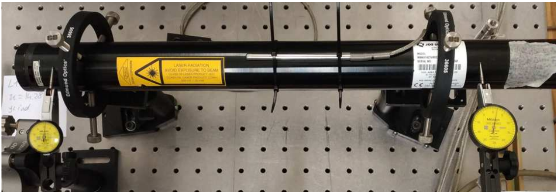
Figure 72. The dial gauges control the position of the He-Ne laser, in the middle, the temperature sensor of the laser.
