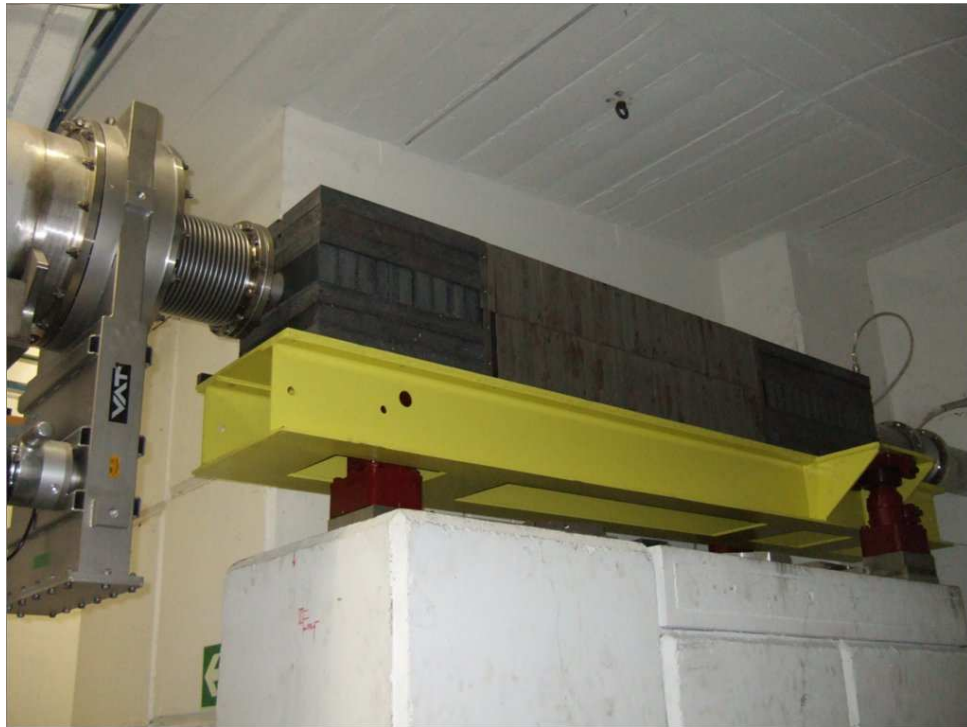
Figure 2.6 – Picture of the beam-shaping collimator located just before the experimental area.
