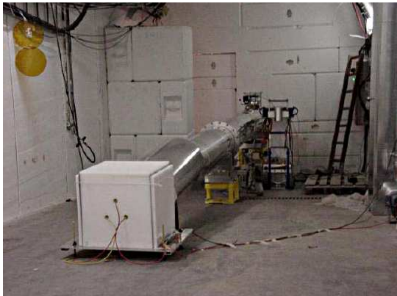
Figure 2.7 – Neutron escape lane area, with the polyethylene block placed at the end of the TOF tube [49].
