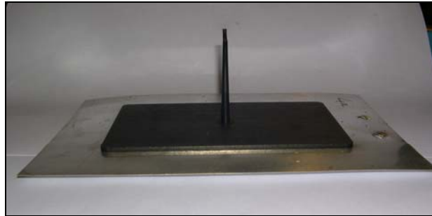
Figure 3.3: Test part (it can be seen the plastic and the metal parts, which are joined together to form the metal-polymer macro-composite, and the freeze sprue of the injection system of the mould).
