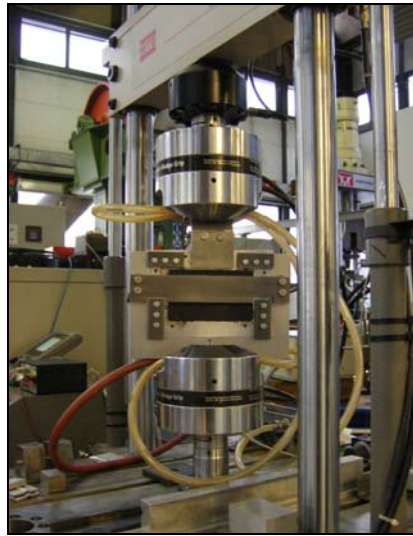
Figure 4.19: Shear test equipment assembled on the MTS machine.
