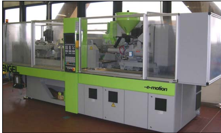
Figure 3.1: The injection moulding machine at DIMEG Lab.
