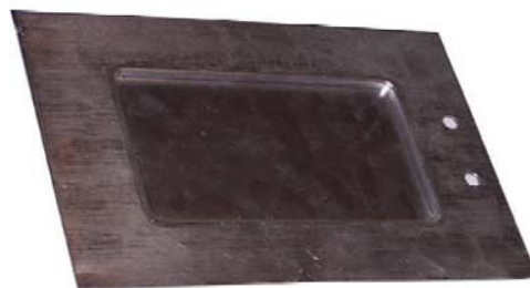
Figure 3.4: Detail of the deformed sheet metal part of the test macro-composite.
