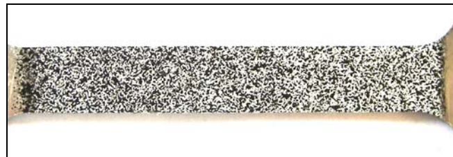
Figure 5.8: Stochastic pattern on specimen surface for tensile tests at high temperature.
