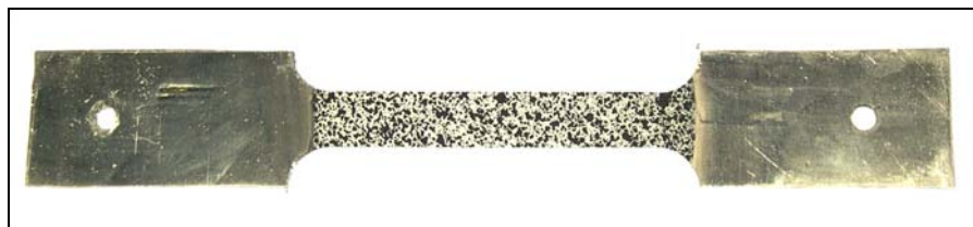
Figure 5.4: Stochastic pattern applied on strain measuring area of specimen.
