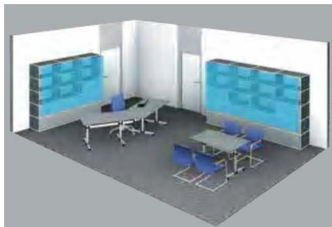
Figure 6-11 Vertical task areas in an office: e.g. “cabinet and shelving system surfaces” (blue) Illuminance value reference height: starting at 0.5 m rising to 2 m above floor level, width according to objects
