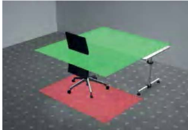
Figure 6-12 Areas defined by DIN 4543: The VDU task area (green) consists of a work surface (white desktop) and a user area (red).
