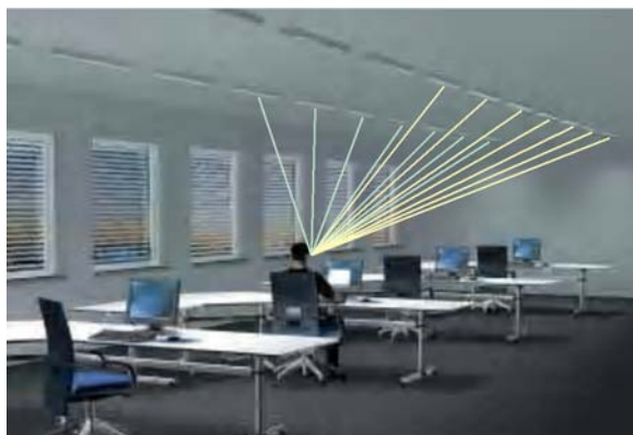
Figure 6-15 The UGR method takes account of all the luminaires in the system which contribute to the glare sensation as well as the brightness of walls and ceilings. It produces a UGR index.
