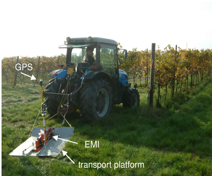
Figure 1 Mobile EC equipment: a) EMI sensor; b) GPS; c) hardware interfacing (hidden inside tractor cabin); d) transport platform.
