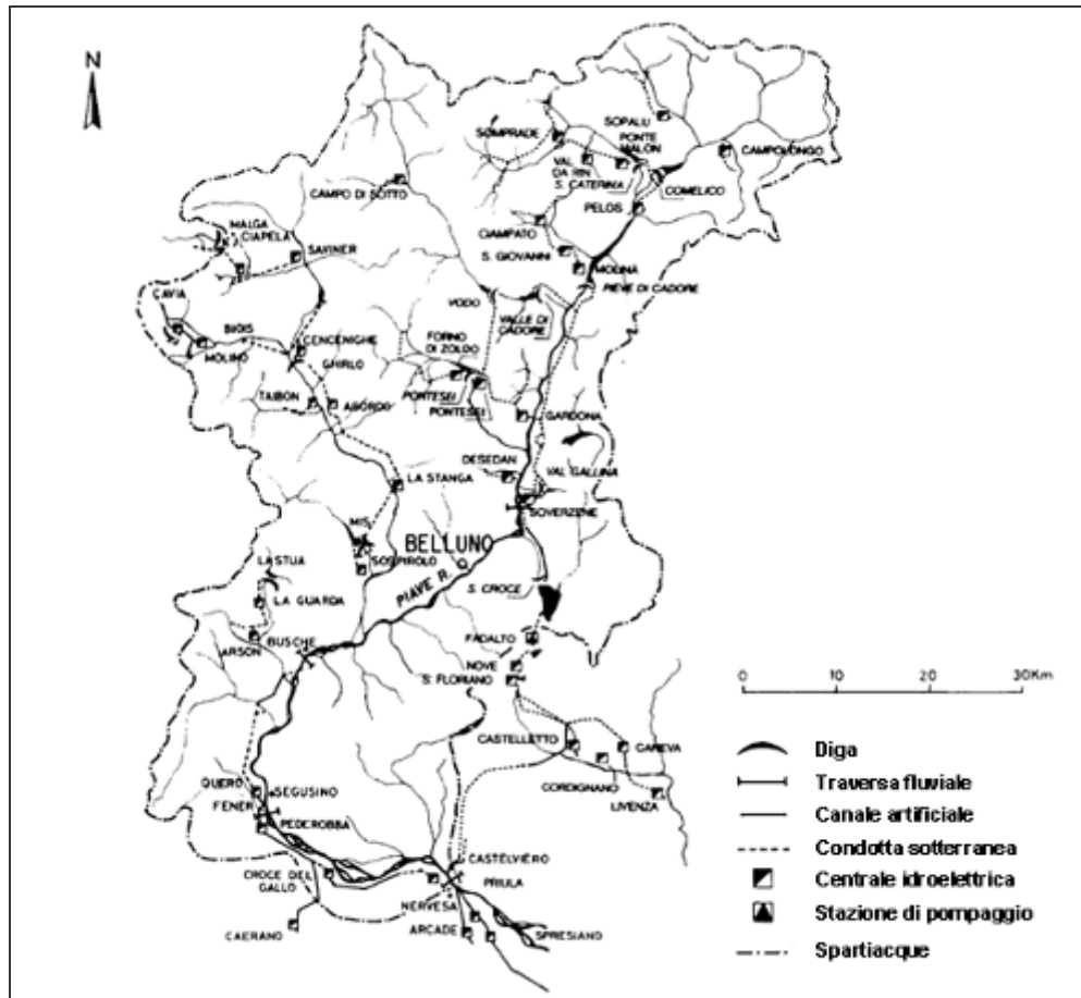
Figure 3.4: outline upon the electric power plants and irrigation works along the Piave river (Surian, 1999)
