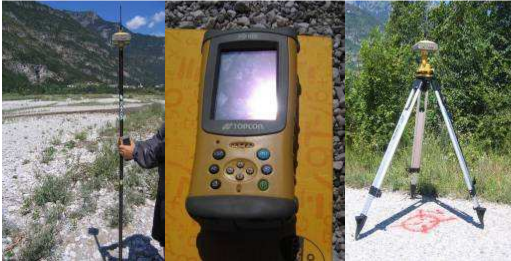
Figure 5.4: differential global positioning system instruments
