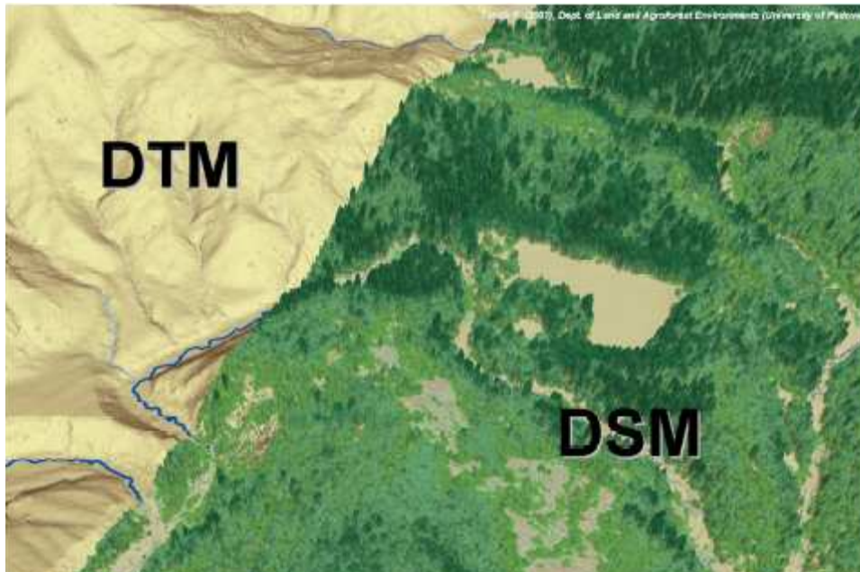
Figure 4.7: differences between DTM (Digital Terrain Model) and DSM (Digital Surface Model) as modified by Tarolli 2007
