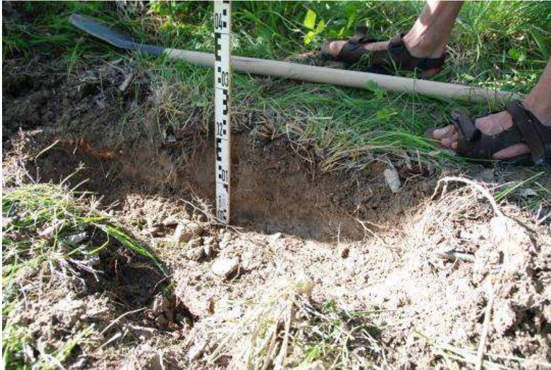
Figure 5.14: fine sediment depth measurements
