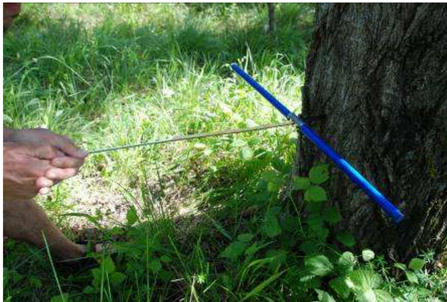
Figure 5.13: sampling with Pressler gimlet
