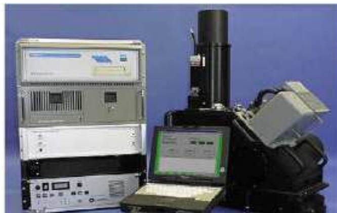
Figure 4.1: AeroScan LIDAR System, showing the Scanner, IMU, and supporting hardware.
