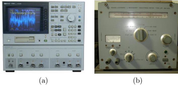
Figure 3.41: (a) HP (Hewlett Packard) 4195A network analyzer, (b) Rohde & Schwart LRT BN6100 inductance meter
