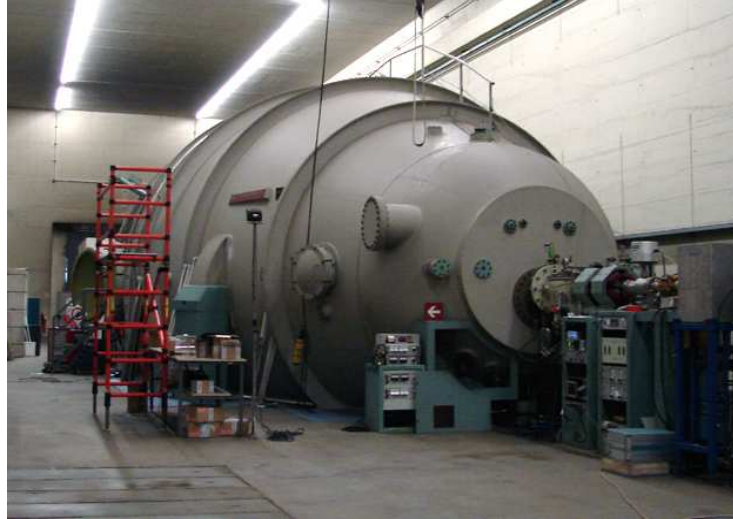
Figure 2.9 The 15MV Tandem XTU at the INFN Legnaro National Laboratories.
