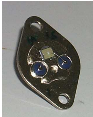
Figure 7.1 MOSFET device ready for irradiation. The die is housed a TO-3 package.
