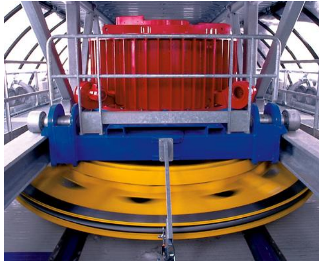
Figure 2.29: SFA direct drive motor of Leitner Ropeways
