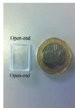
Fig. 2.5. Image of the quartz cuvette with two open ends.
