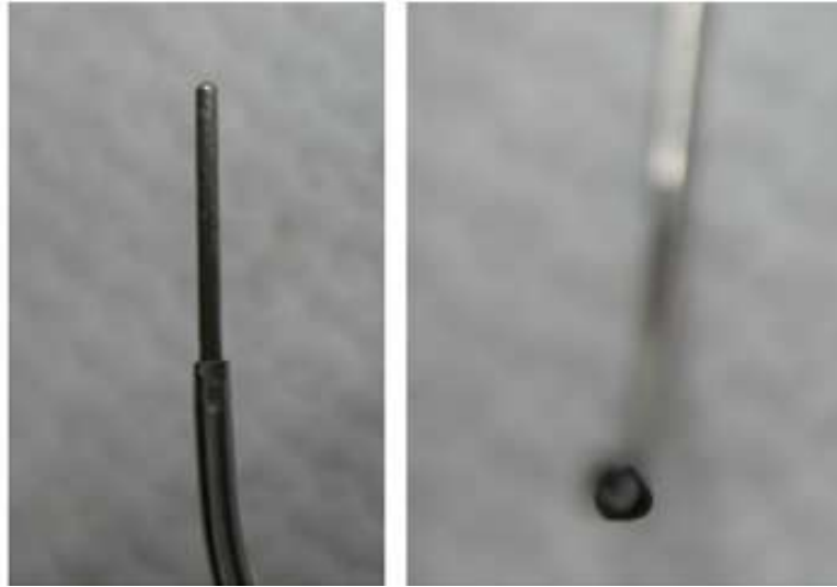
Figure 6.9: Thermocouples crimped to stainless steel pipe (left); expansion of the tip (right).
