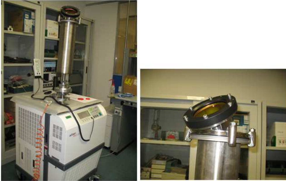
Figure 7.22: Set-up for the vacuum tightness of the infrared camera window.
