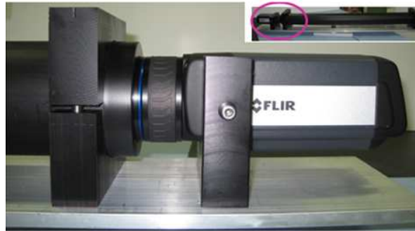
Figure 6.33: Thermal camera installed on the tube.
