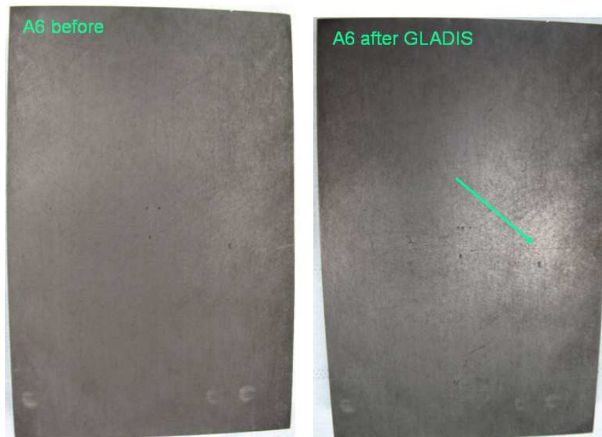
Figure 7.81: A6 rough side, before and after exposure to the GLADIS beam.
