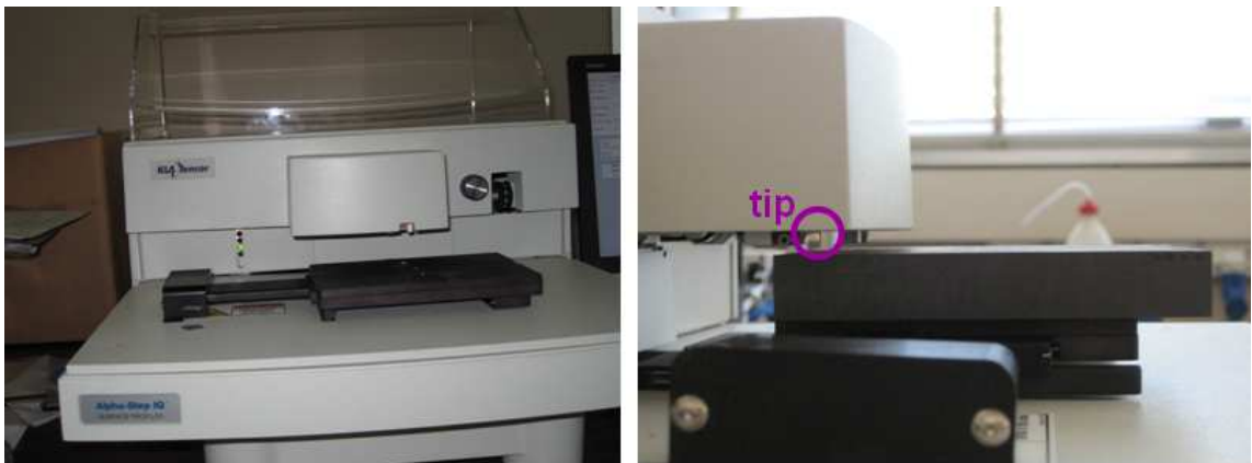
Figure 4.4: profilometer device (left hand side) and test on prototype (right hand side).
