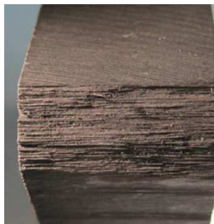
Figure 2.2: CFC: the fibres are arranged along the thickness.
