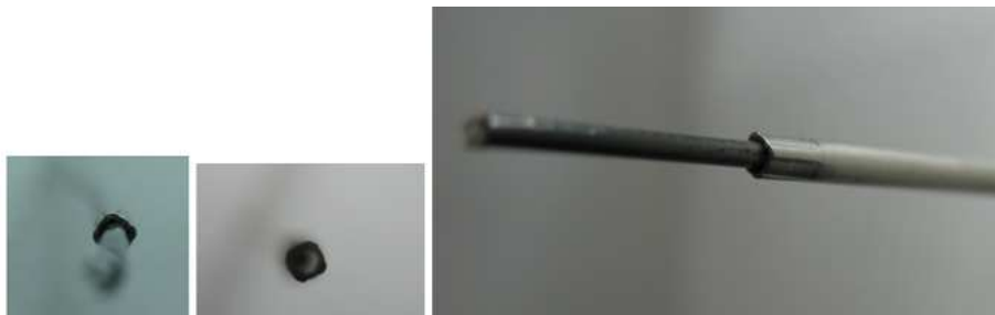
Figure 6.24: Thermocouple crimped in 4 points.
