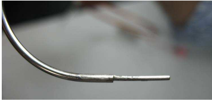
Figure 6.7: Thermocouples braze welded to stainless steel pipe.
