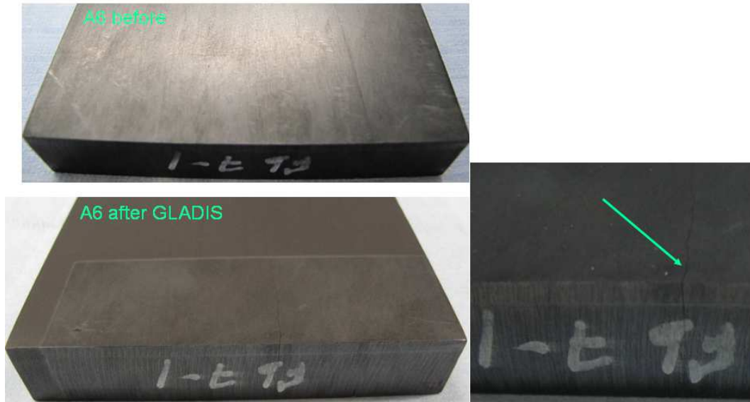
Figure 7.80: Details of crack in A6 smooth side.
