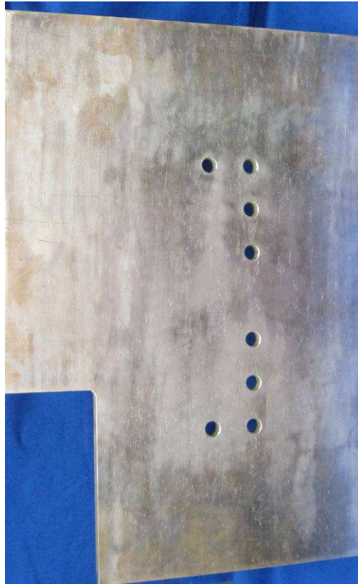
Figure 7.6: Mask to create beamlet geometry.
