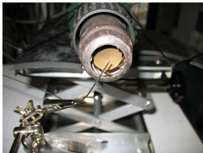
Figure 6.15: Measurement of the temperature of the air blower.
