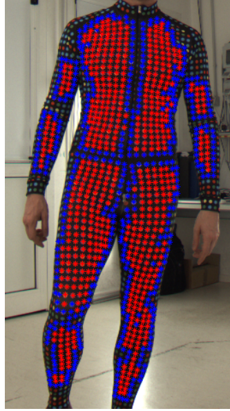
Figure 3.1.24: ID added thanks to the garment map. Red asterisks indicate marker for which the ID is calculated relying on the colours of the neighbours. Blue asterisks indicate markers that receive an ID thanks to the neighbours ID and the map
