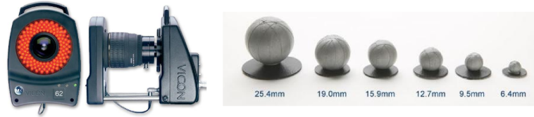
Figure 3.5.3: Left: Vicon camera with active IR illumination. Right: Spherical retro-reflective markers with different sized.
