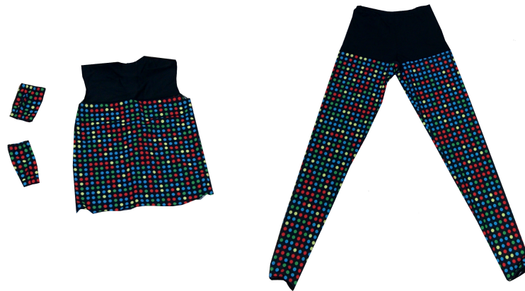
Figure 5.1.1: Veritas 4 pieces suit. Left: 3 pieces suit used for upper limb analysis. Right: trousers for lower limb analysis.
