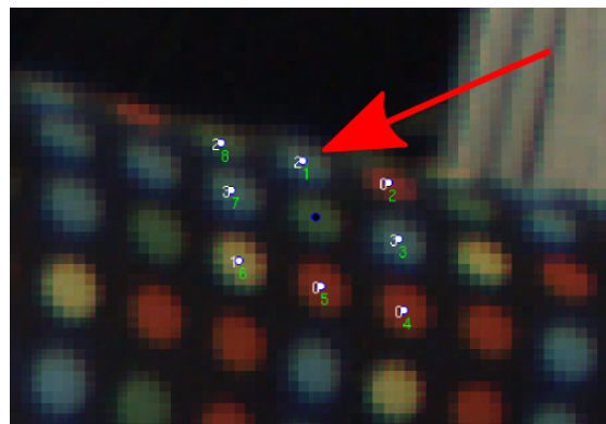
Figure 3.1.20: Wrong marker color association. The arrow indicates the markers that is classified as a green marker (label=2) instead of a blue marker (label=3). The numbers in white are the color-labels of the each marker. The numbers in green indicate the order in which they marker should be read to generate the ID.
