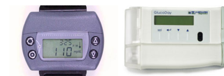
Figure 1.6: GlucoDay ® S device: receiver (left) and transmitter (right) attached to the inserted sensor [35].
