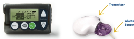
Figure 1.5: The Guardian ® REAL-Time [32]. REAL-Time CGM System monitor (left), the MiniLink REAL-Time Transmitter together with the glucose sensor inserted in the subcutis (right).
