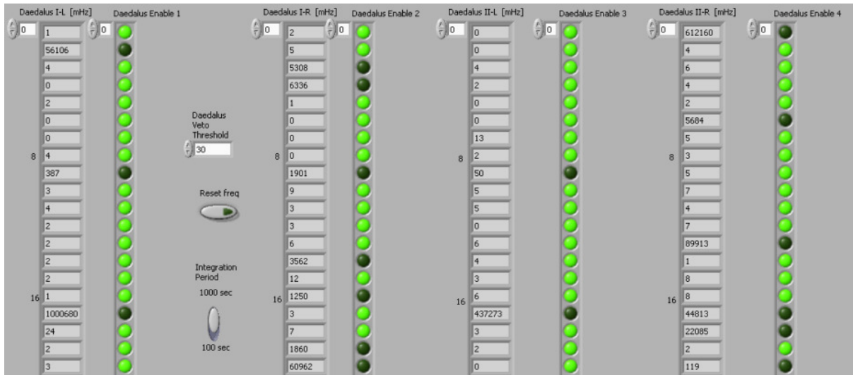
Figure 5.2: View of the main trigger interface. All the trigger rates for SD in collection views are displayed in mHz, while the veto is represented by the array of LED. The control for setting the threshold of the automatic veto is also shown.
