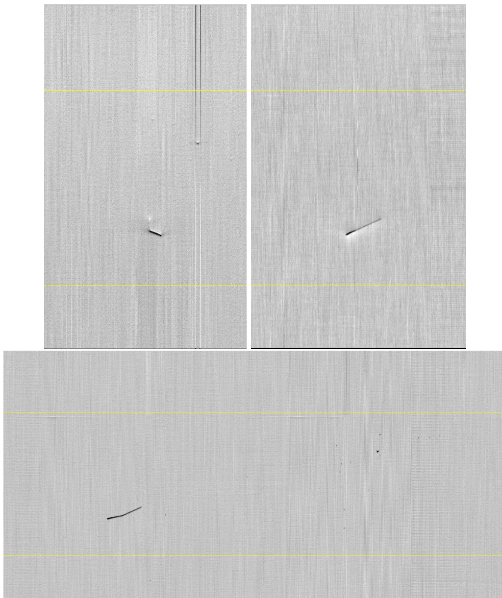
Figure 5.4: Neutral event triggered by CNGS gate + Super Daedalus. The three views, Induction1 (top left), Induction2 (top right), Collection (bottom), are shown: the yellow lines represents the detector volume.
