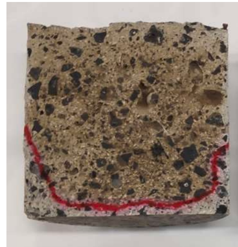
Fig. 13. Chloride footprint in 28 days in a specimen of mix SC/II.
