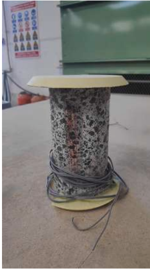
Fig. 4. Faced and instrumented core.
