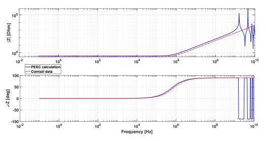
**Figure 22.** Frequency response of the excitation coil impedance calculated with the PEEC filamentary model (solid blue line) and with resistance and inductance parameters estimated in Comsol (dashed-dotted red line).
