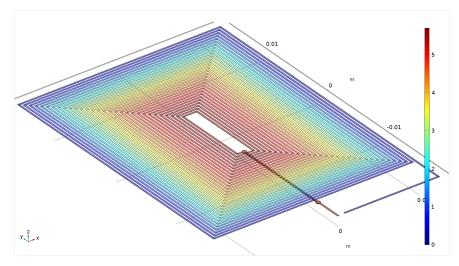
Figure 9. Calculated voltage distribution for the surface current model, expressed in V.
