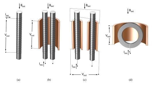
**Figure 2.** Parallel fluxgate configurations. (**a**) Single-core, (**b**) Vacquier, (**c**) Förster, (**d**) Aschenbrenner, and Goubau (ring-core); in gray is the ferromagnetic core and the detection winding is in orange when separate from the excitation.
