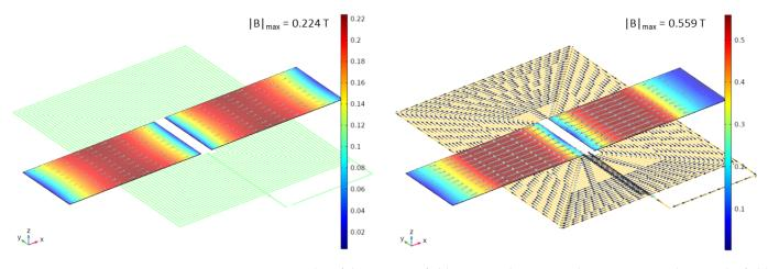
**Figure 10.** Contour-plot of the magnetic field norm on the cores with gray arrows indicating the field direction, together with contour-plot of the current density norm on the excitation coil with black arrows indicating the current direction, at t = 0 s (**left**) and  $t = 25 \,\mu$ s (**right**) corresponding to zero and the peak current, respectively, for a 150  $\mu$ T external field. Color bars in T.
