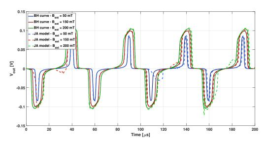
**Figure 13.** Differential output voltage calculated by adopting the parameters related to the JA1 loop (dotted lighter lines), for three values of the external magnetic field (50, 150, and 200  $\mu$ T), compared to the related ones calculated with the corresponding BH characteristic (continuous darker lines).
