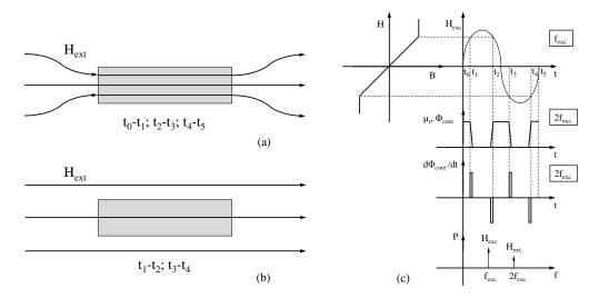
**Figure 1.** Scheme of the basic fluxgate working principle. (a) The core is not saturated, and the magnetic flux is concentrated inside. (b) The flux is "gated" out when the permeability drops to  $\mu_0$ . (c) Time evolution of the main quantities in a period of the excitation field  $H_{exc}$ .
