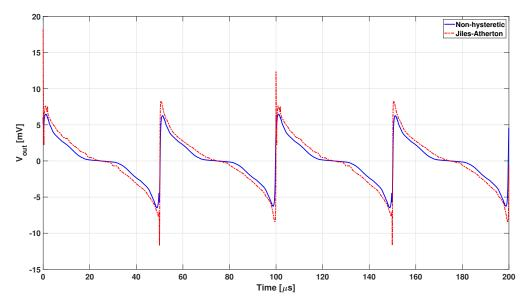
**Figure 17.** Output voltage obtained with the hysteretic Jiles–Atherton model with the JA1 parameters for an external magnetic field of 100  $\mu$ T (red dashed-dotted line), compared to the one calculated in the same condition with non-hysteretic B-H curve (solid blue line).
