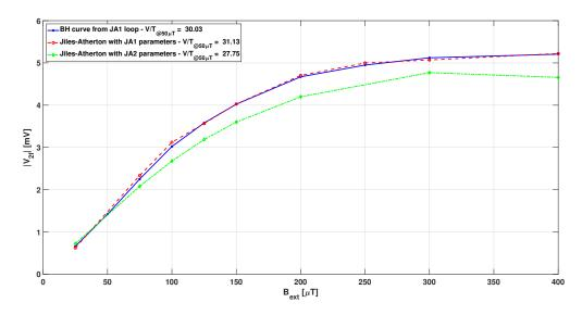
**Figure 19.** Second harmonic of the output voltage against the related external magnetic field for the different analyzed cases: non-hysteretic JA1 model (solid blue), hysteretic JA1 (dashed red), and JA2 (dahed-dotted green) model.
