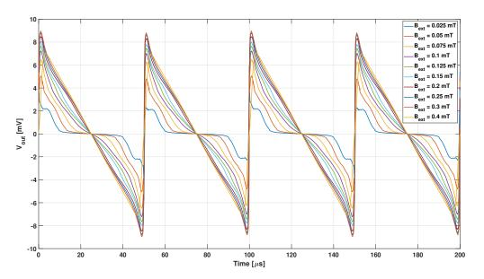
**Figure 16.** Output voltage obtained with the non-hysteretic B-H curve from JA1 material model for different values of the external magnetic field.
