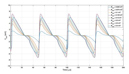
**Figure 18.** Output voltage obtained with the hysteretic Jiles–Atherton model with the JA2 parameters for different values of the external magnetic field.
