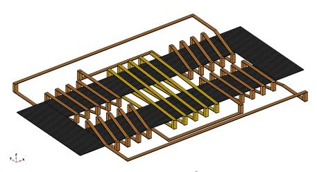
**Figure 15.** Meshed model implemented in Comsol<sup>®</sup> reproducing the MSFS sensor described in [25] Copyright 2022 Elsevier; in gray is the ferromagnetic core, the excitation coils are in orange, and the detection coil is in yellow.
