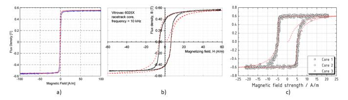
**Figure 5.** Fitted hysteresis loops (dashed red lines) overlapped to the original images for the cases named JA1, JA2, and JA3, respectively, in (**a**–**c**).
