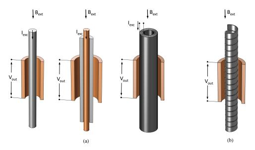
**Figure 3.** Orthogonal ((**a**) Aldredge) and mixed-mode ((**b**) Schonstedt) fluxgate configurations; in gray is the ferromagnetic core, and detection winding and solid excitation conductor are in orange (if present).
