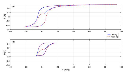
**Figure 20.** Hysteresis loop covered in one excitation period by the left (solid blue lines) and right (dashed red lines) core legs with the closed core configuration (**a**) and with a 0.5 mm air gap (**b**), when an external field of 100  $\mu$ T is applied, and the JA2 hysteresis model parameters are used.
