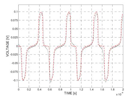
**Figure 11.** Calculated differential output voltage with 150  $\mu$ T external field (dashed-dotted red line) overlapped with the experimental results from Figure 13 in [33] (Copyright 2022 IEEE Transactions on Instrumentation and Measurement) obtained in the same conditions.
