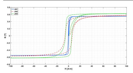
Figure 6. Comparison of the hysteresis loops reconstructed from the Jiles–Atherton parameters of fitted curves JA1 (continuous blue), JA2 (dashed red), and JA3 (dash-dotted green) reported in Table 2.
