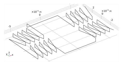
Figure 21. Filamentary model of the excitation oil used to calculate its frequency response.
