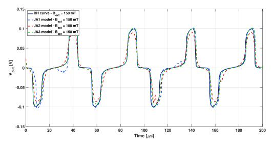
**Figure 14.** Differential output voltage calculated adopting the Jiles–Atherton model for the JA1, JA2, and JA3 loops (dotted lighter lines) with external magnetic field of 150  $\mu$ T), compared to the one calculated without hysteresis (continuous darker lines).
