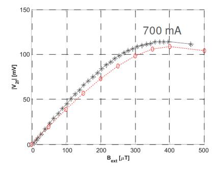
**Figure 12.** Second harmonic of the calculated differential output voltage plotted against the related external magnetic field (dashed red line and circles), overlapped to the experimental results from Figure 14 in [33] Copyright 2022 IEEE Transactions on Instrumentation and Measurement.
