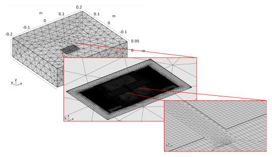
**Figure 8.** Mesh implemented for the PCFS model: the overall dimension of the air volume and different levels of detail (in red boxes) are shown.
