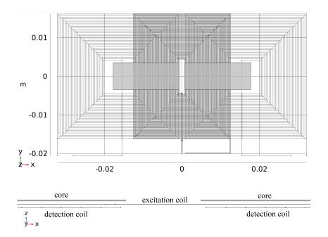
**Figure 7.** Implemented geometrical model reproducing the PCFS type sensor described in [33] Copyright 2022 IEEE Transactions on Instrumentation and Measurement; top view on the top and zoomed side view at the bottom of the figure.
