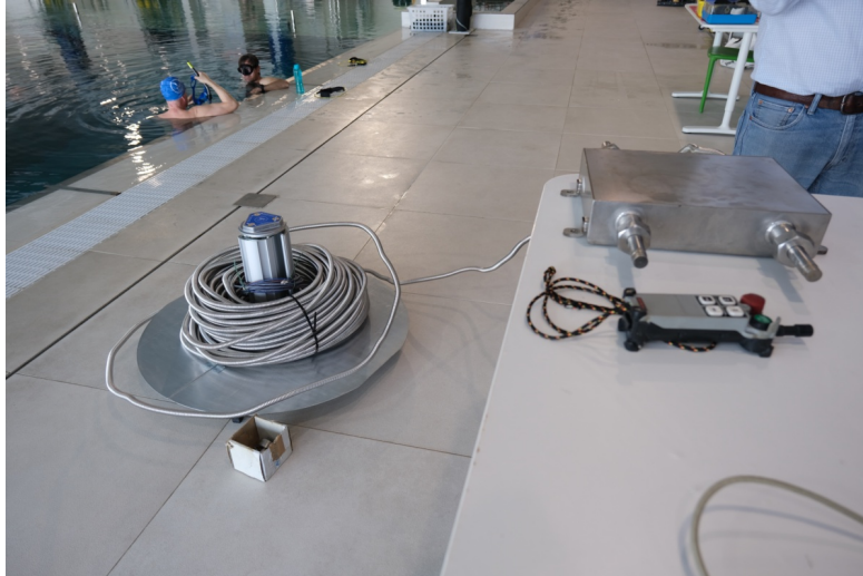
Figure 9.13: UWB with its bellow cable twisted in the uncoiling system.
