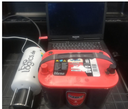
Figure 4.5: Picture of the apparatus used in the experiment. Each node was equipped with batteries, a laptop and an acoustic modem.
