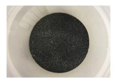
Figure 7: Appearance of the diluted bed after the two TPR-TPO cycles.
