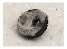
Figure 4: Spent CuO bed after 11 redox cycles.
